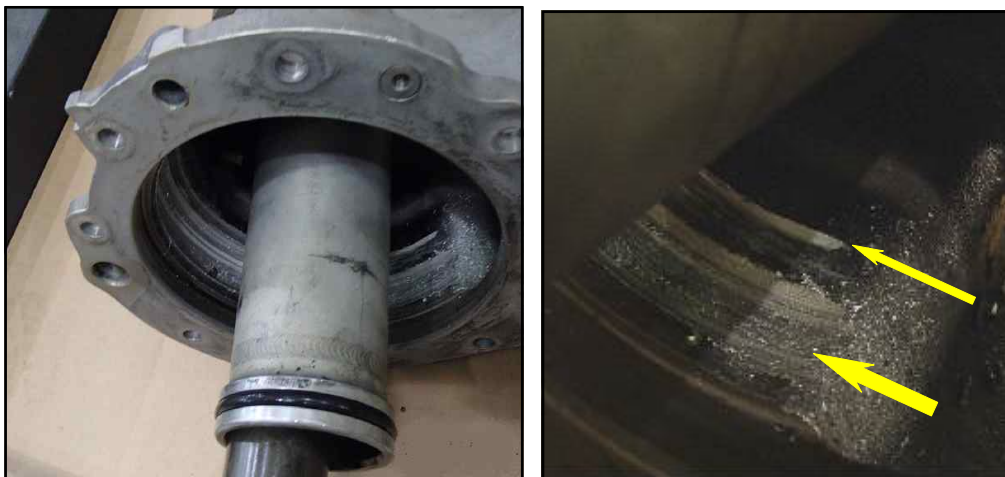
[Figure 9] Damaged Gearbox Driveshaft Front Housing
