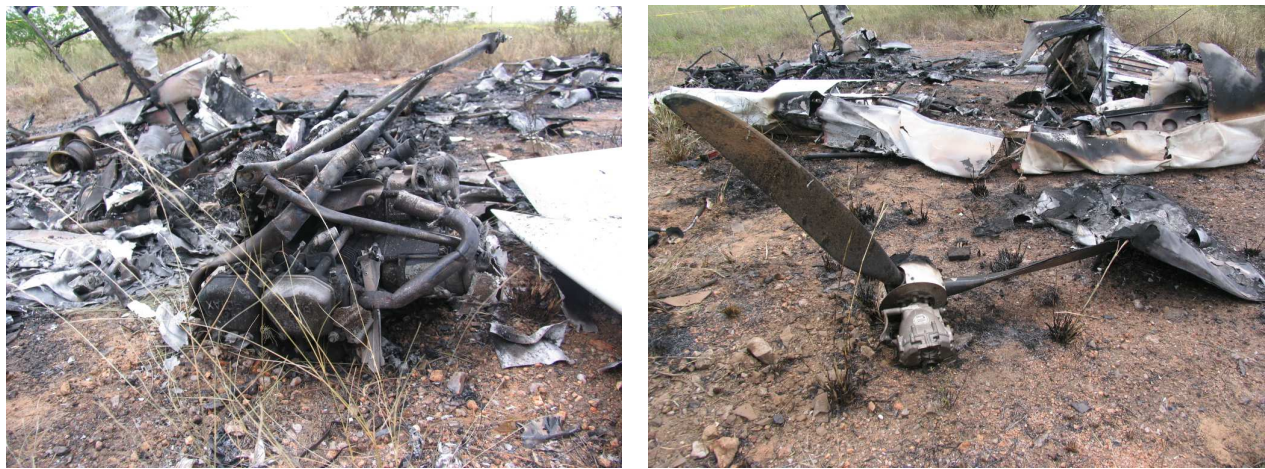
Figure 8. A view of the engine as it came to rest (a) and the propeller with two of the three blades still attached (b).
