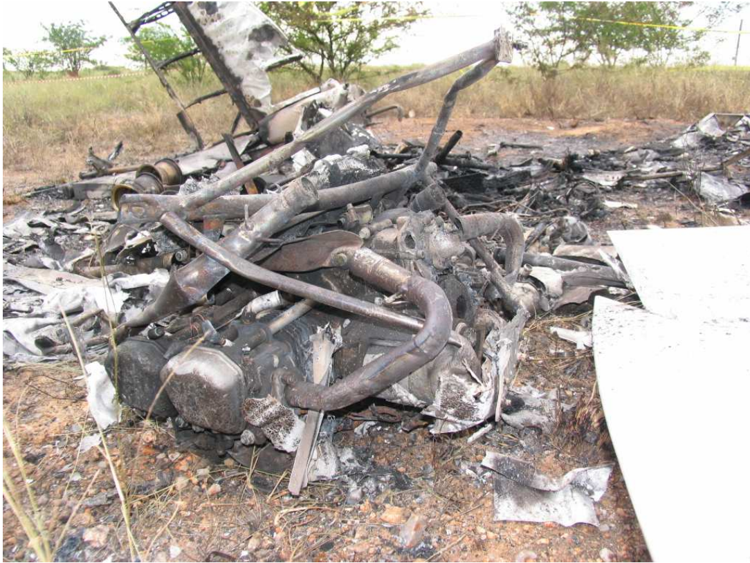
A photo of the engine that was taken on the scene of the accident lying in an inverted attitude.
