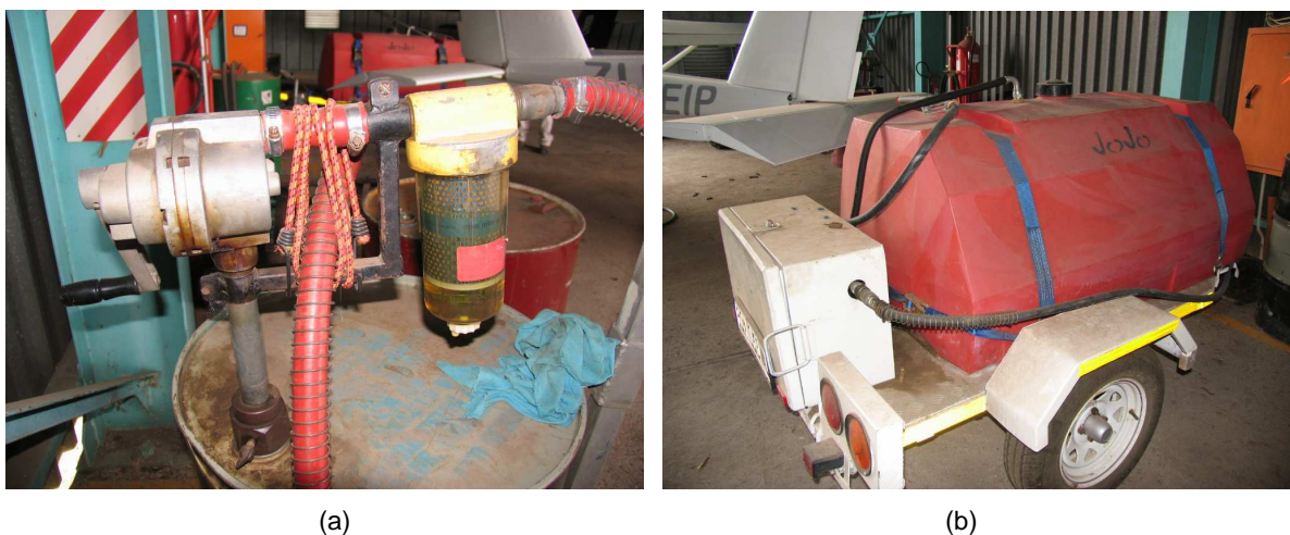
Figure 5. A view of a 200 litre drum with a hand crank device (a) as well as a trailer type bowser in the hangar (b).
