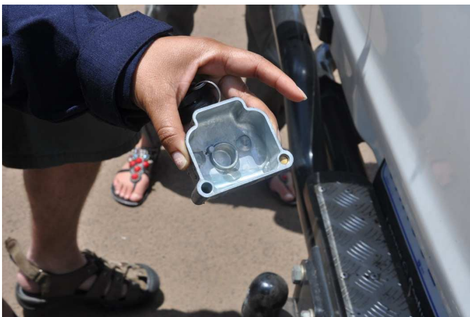
Figure 9: Carburettor at accident site did not contain any oil.
