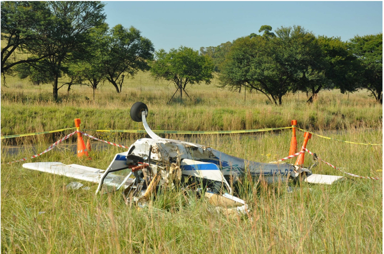
Figure 3: Damage sustained to the fuselage, undercarriage, propeller, engine and wings.
