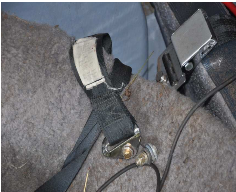
Figure 7 & 8: The pilot's seat belt that became dislodged from the aircraft on impact
