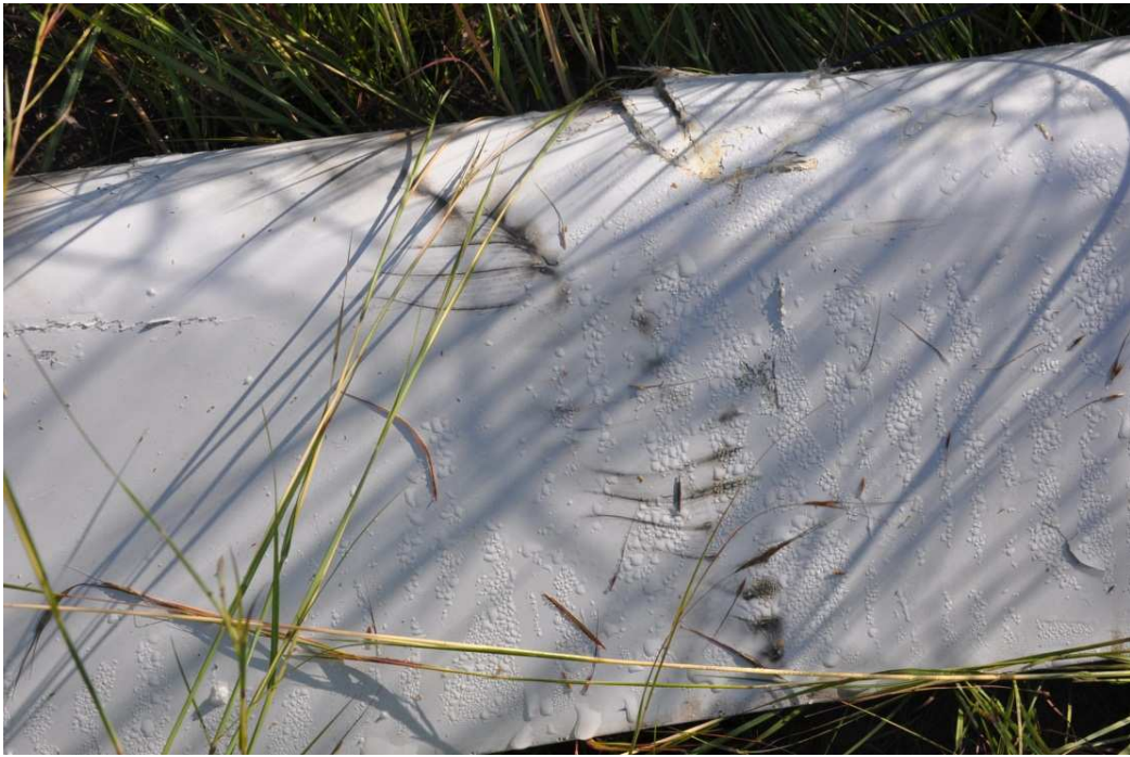
Figure 6: Evidence of arcing close to the trailing edge of the aircraft's right hand wing
