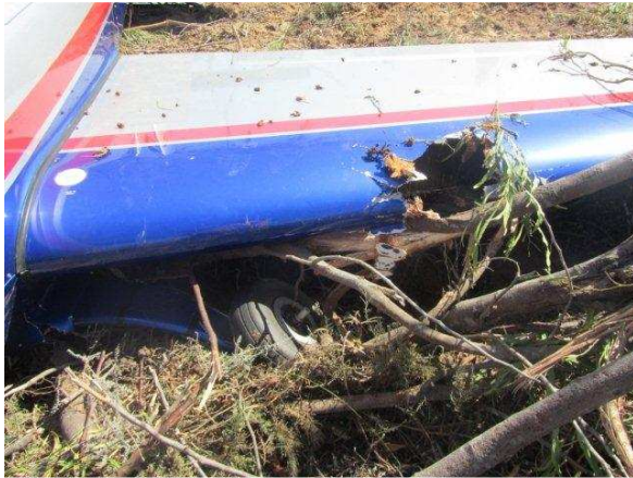
Fig 1: Damage to wing and undercarriage
