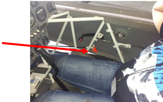
Fig. 5 Location of the fuel selector from the pilot seat
