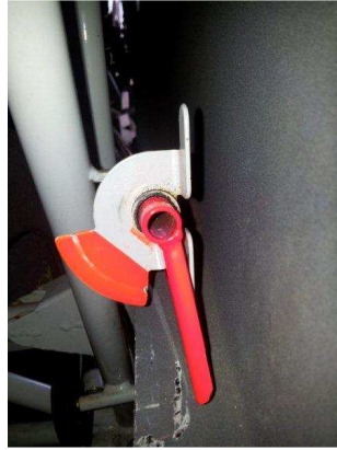
Fig. 7 Fuel selector in the OFF position
