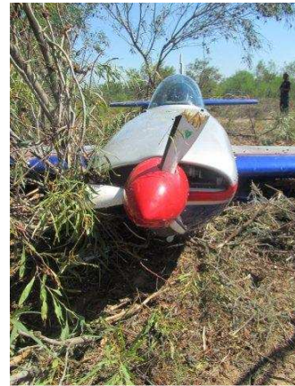
Fig 2: Damage to the propeller
