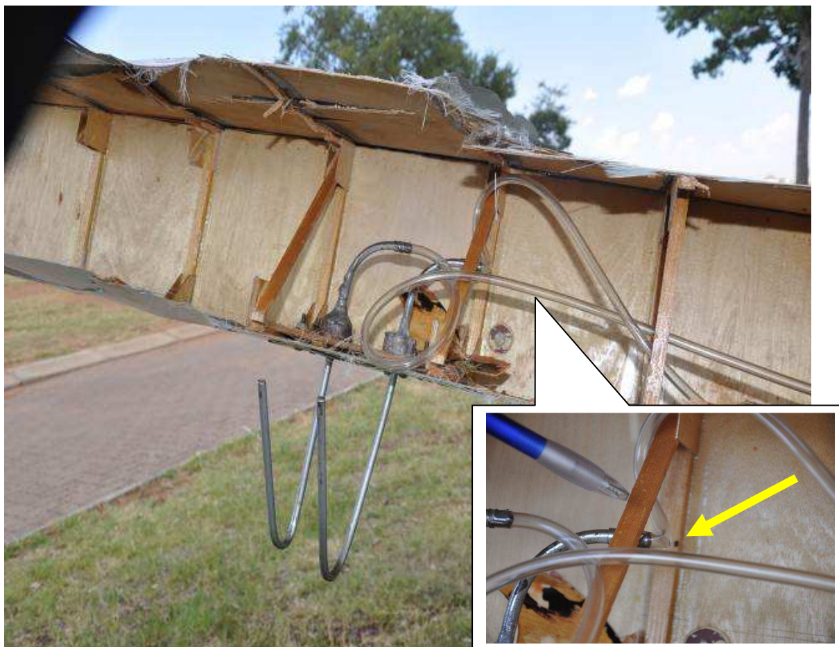
Figure 6: View of the incorrectly installed static line
