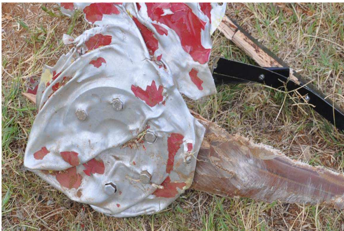
Figure 5: View of the propeller and witness marks on it
