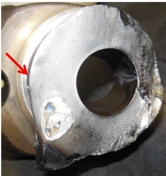
Figure 6 & 7: Fracture showing initiation point and scoring damage aft and forward
