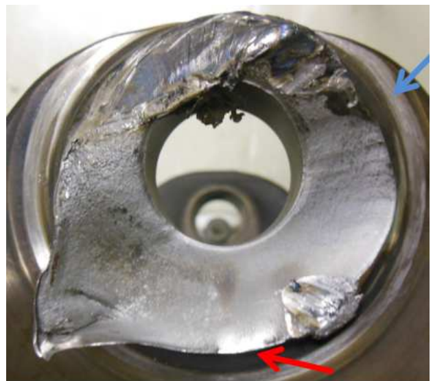
Figure 6 & 7: Fracture showing initiation point and scoring damage aft and forward
