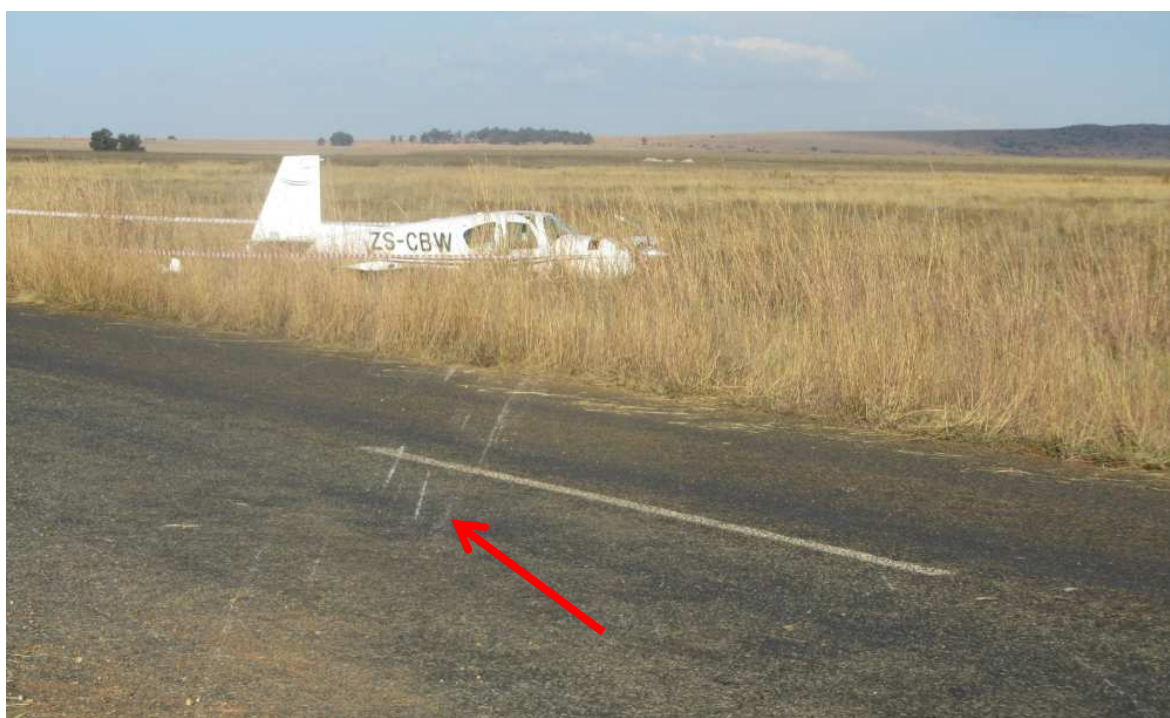
Figure 3: Indicates the skid marks across the road made by the aircraft prior to coming to rest.
