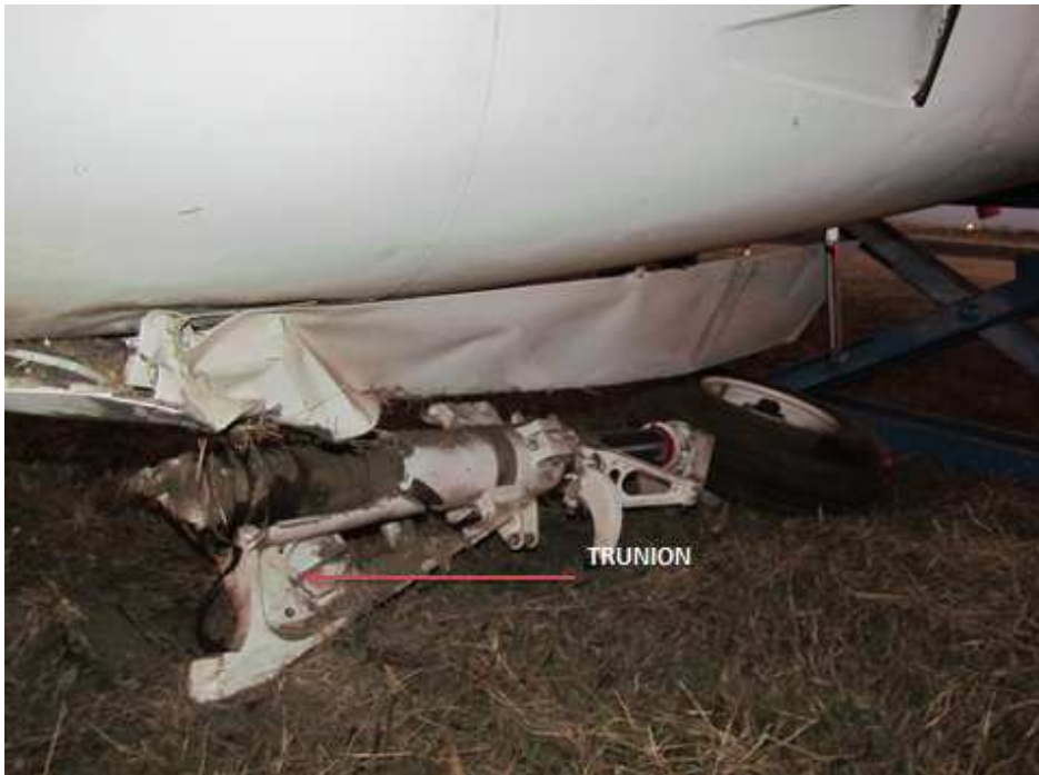
Figure 6, shows the broken nose landing gear trunion
