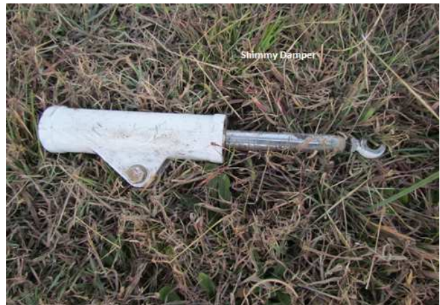
Figure 7 and 8, shows the nose landing gear debris (steering collar and the shimmy damper).
