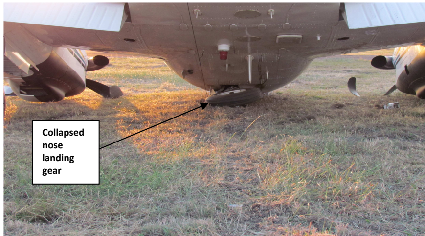
Figure 3, shows damage to nose landing gear of the aircraft.
