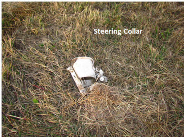
Figure 7 and 8, shows the nose landing gear debris (steering collar and the shimmy damper).
