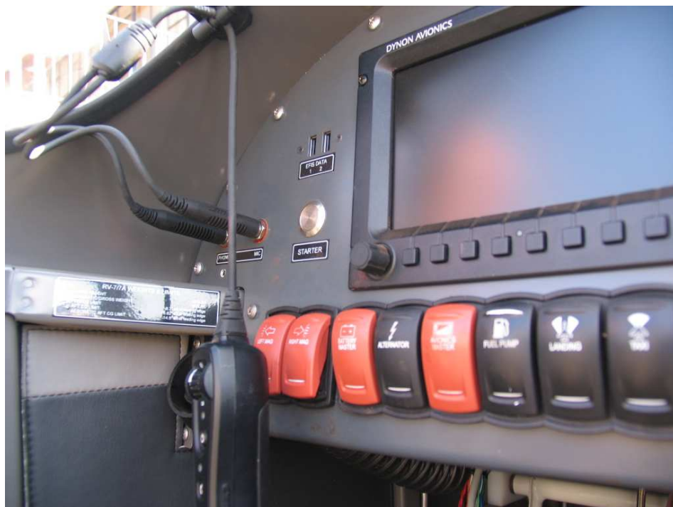
Figure 10. The photo displays the headset control mechanism with the magneto switches in the ON position.
