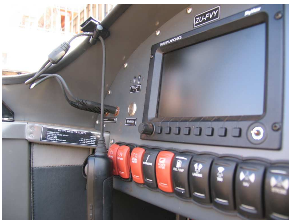
Figure 11. The photo displays the headset control mechanism with the magneto switches in the OFF position.
