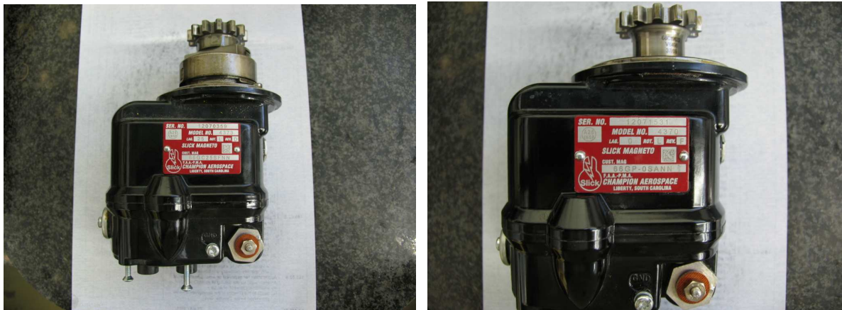
Figure 15. A view of the two magnetos after they were removed from the engine prior to bench testing.
