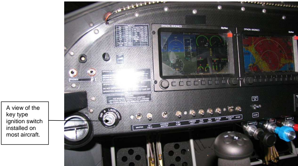
Figure 5. A view of the layout of the switches that was opted for by another owner, similar type of aircraft.
