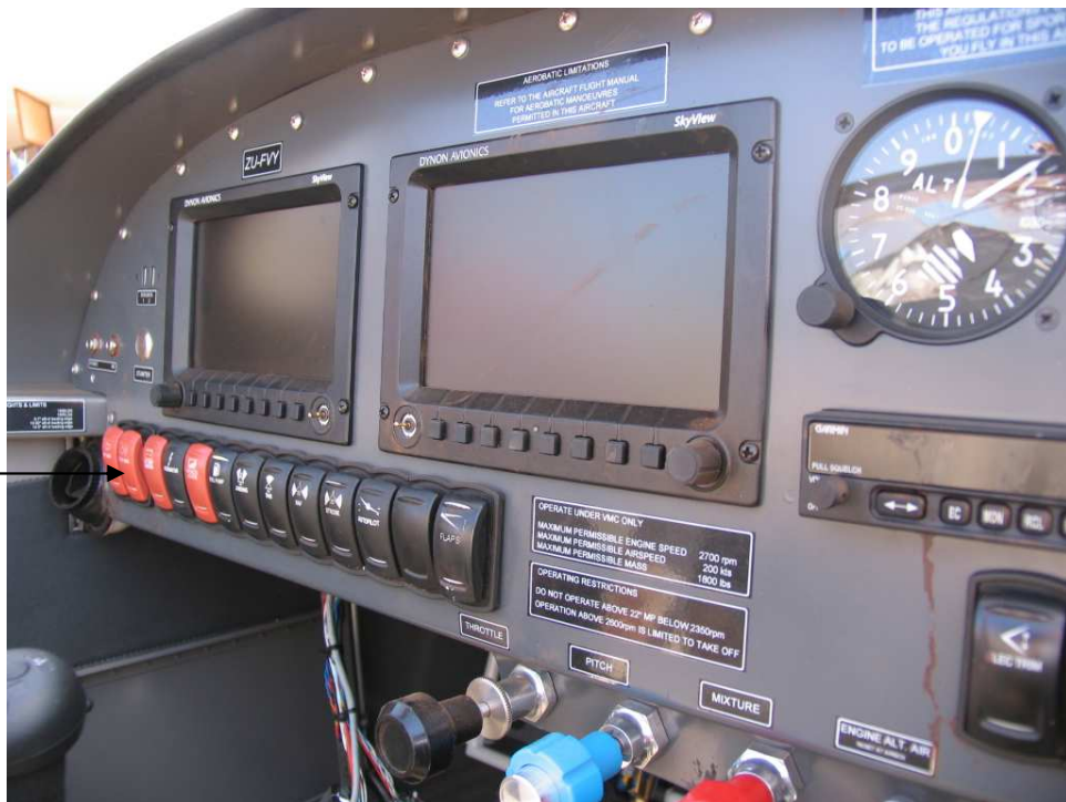
Figure 3. A view of the layout of the switches that was opted for by the owner/pilot of ZU-FVY.
