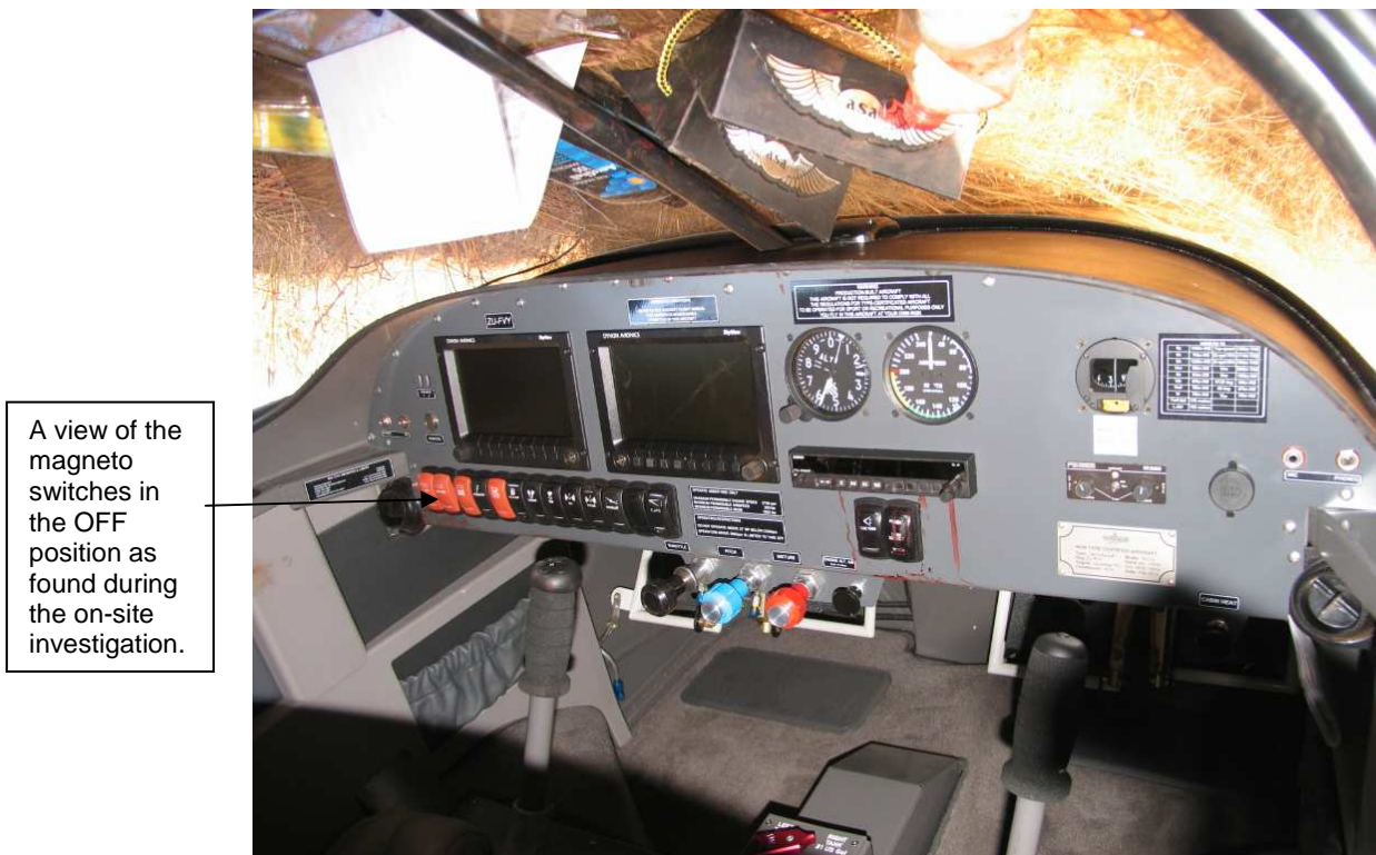
Figure 8. A photo of the cockpit, which was taken during the on-site investigation, aircraft in an inverted attitude.
