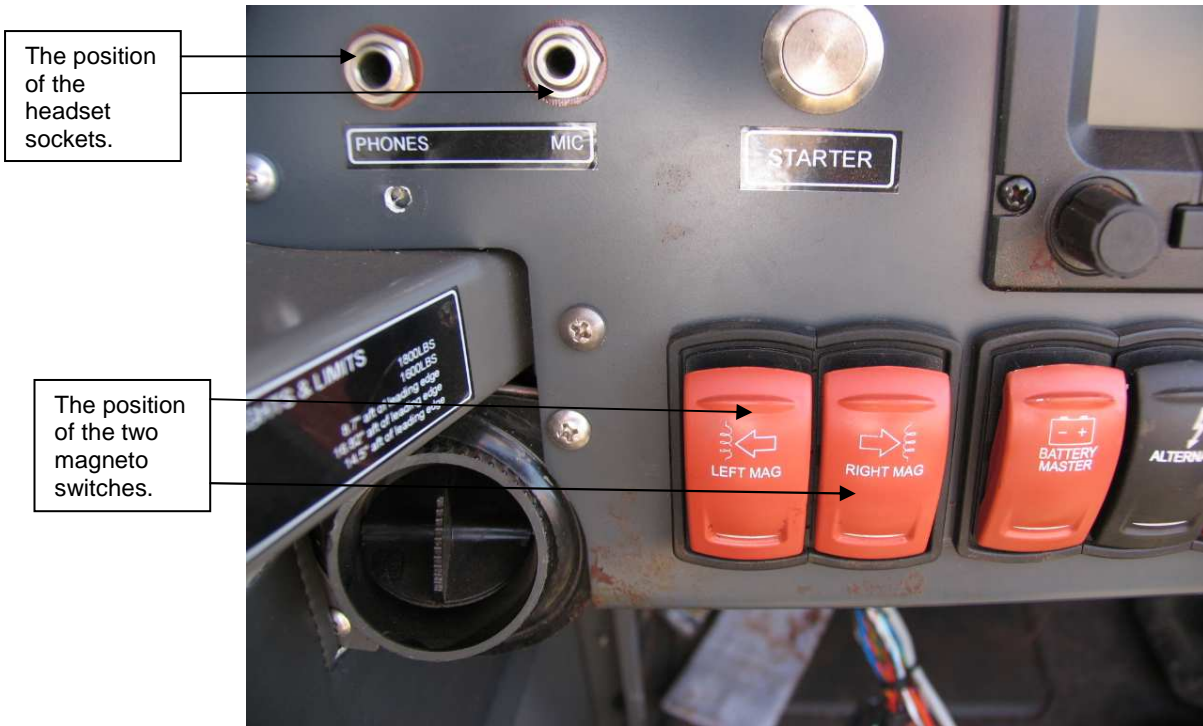
Figure 4. A close-up view of the two magneto switches as well as the battery master switch on ZU-FVY.
