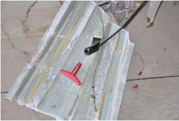
Figure 10: The activation T-handle in the slack position
