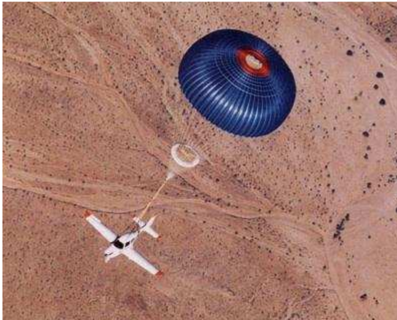
Figure 17: View of CAPS deployed
