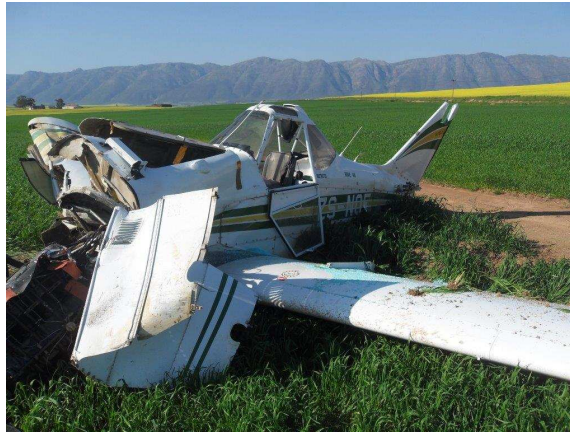
Figure 5: The destroyed forward section of the aircraft
