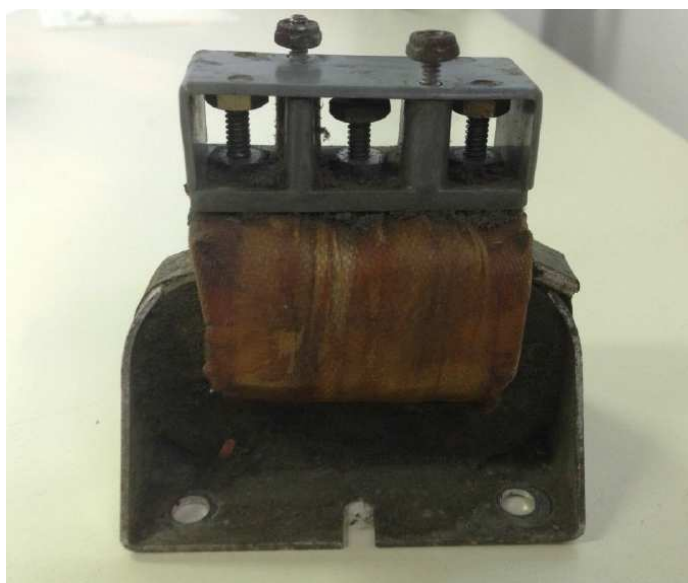
Figure 5: The T98 transformer that was removed from the aircraft.
