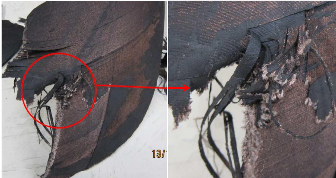
Figure 2: Sharp cut on the No.2 tire piece
