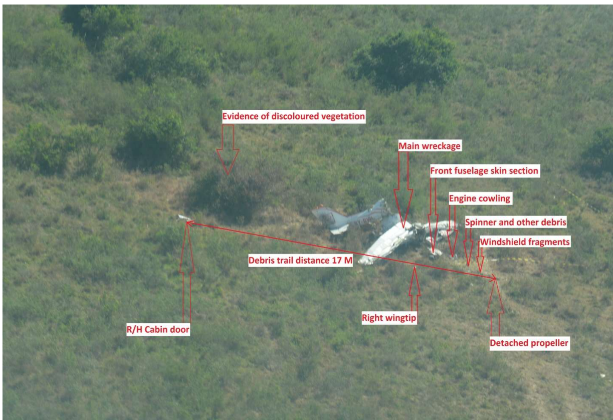
Figure 2: Wreckage debris trail at the accident site
