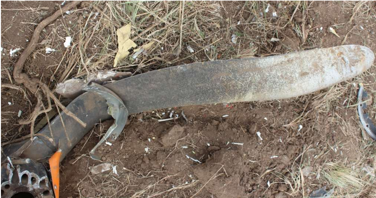
Figure 22: Propeller blade close-up indicating damage
