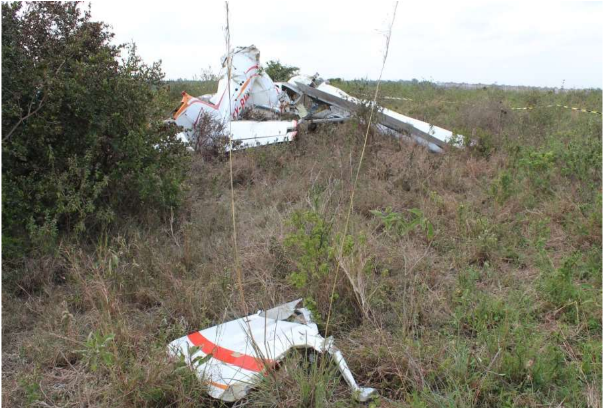
Figure 16: Right cabin door and main wreckage as seen from the rear section of the aircraft
