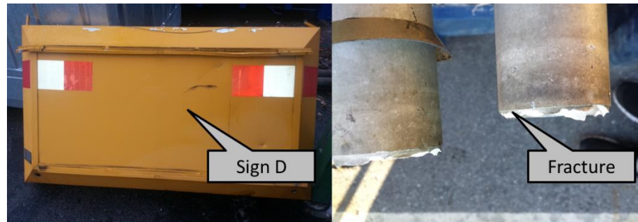
Figure 4. Sign D incl. fracture surface of legs. Photo: Swedavia.
