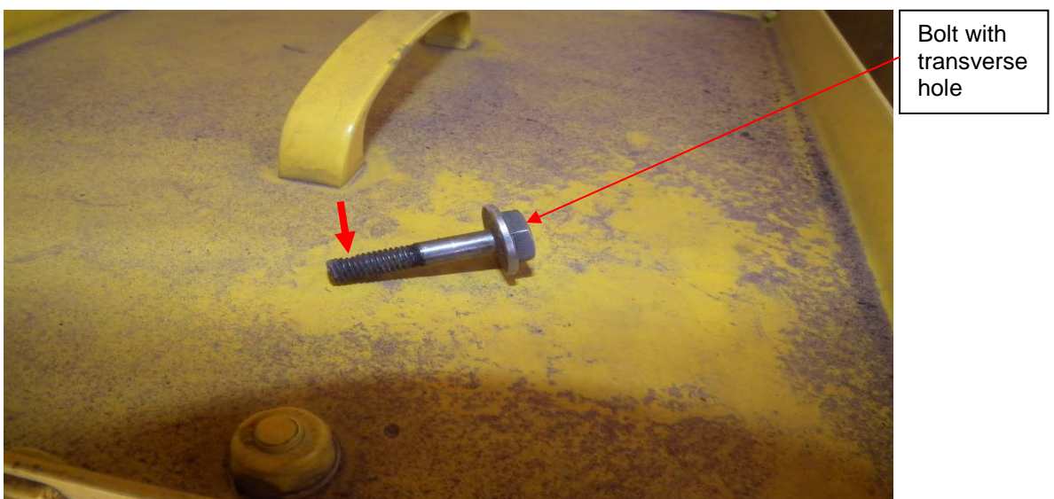
Figure 8: View of the bolt that was found inside the engine cowling.
