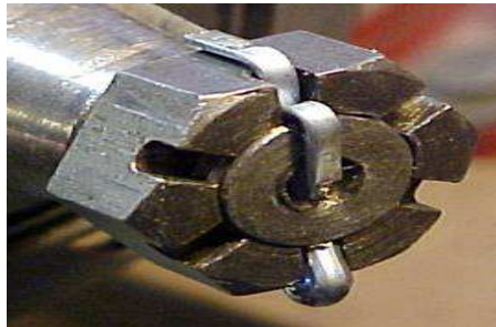
Figure 9: Locking of a castellated nut on bolt .
