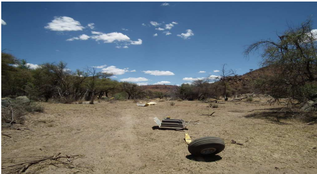
Figure 5: Position of the right gear and debris as found at the accident site.
