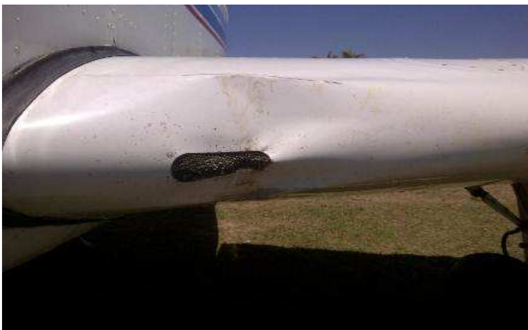
Figure 1: Damage to wing
