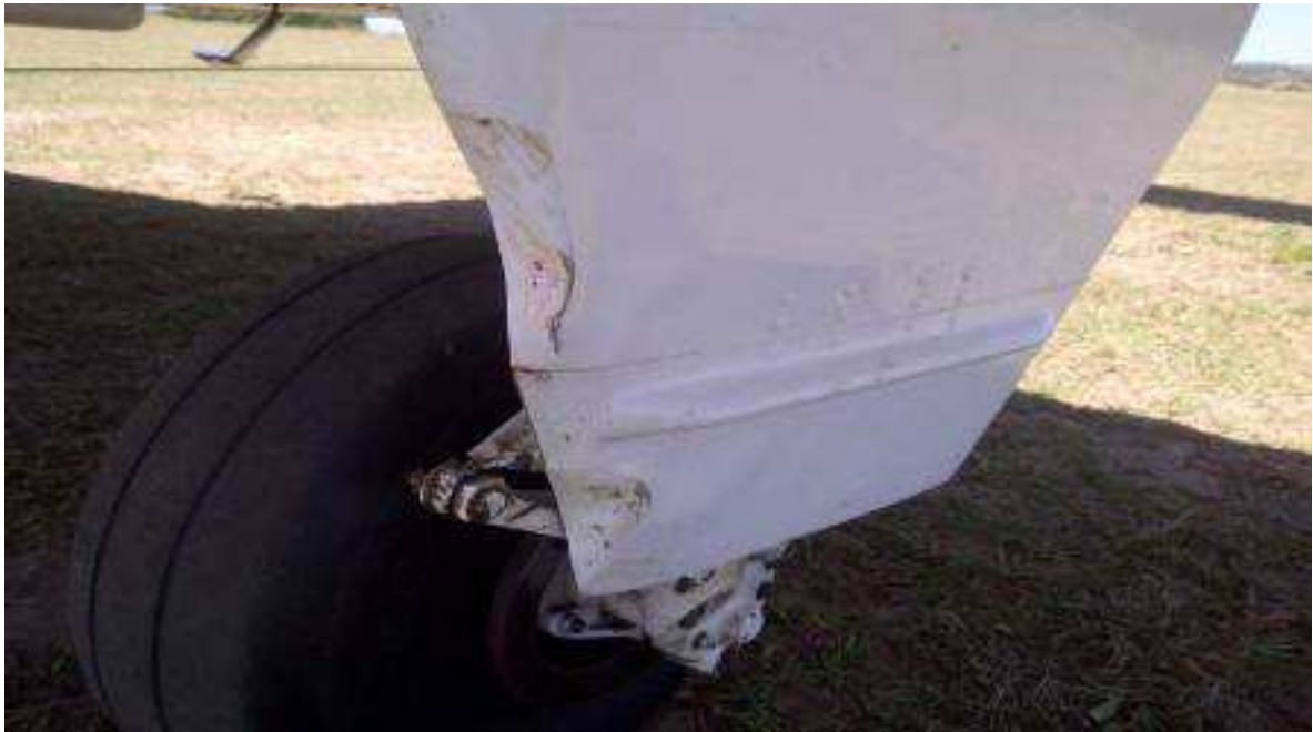
Figure 2: Damage to landing gear door
