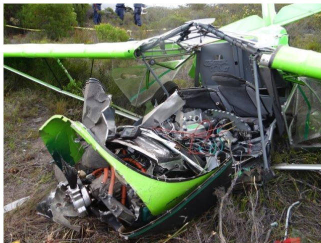
Figure 7: The destroyed forward section of the aircraft
