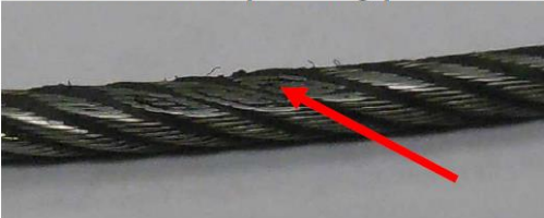
Photo 6: Mechanical abrasive wear evident at other cable positions (digital)
