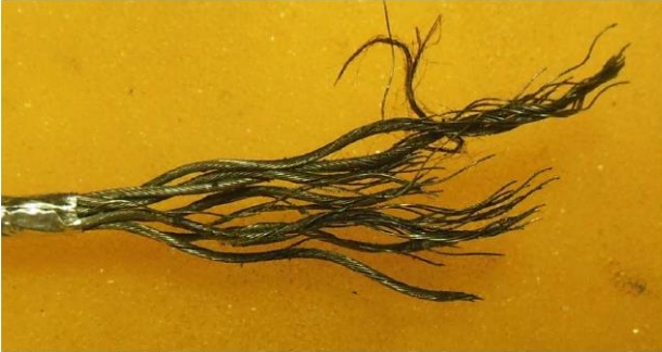
Photo 4: Fractured right hand cable (digital)
