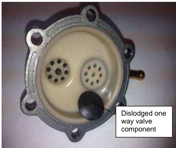
Figure 7: Dislodges one-way valve
