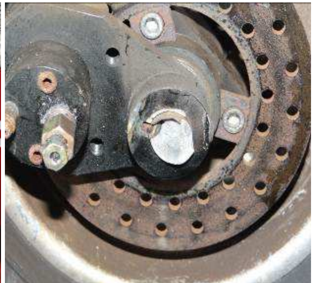
Figure 5: Left main wheel broken off
