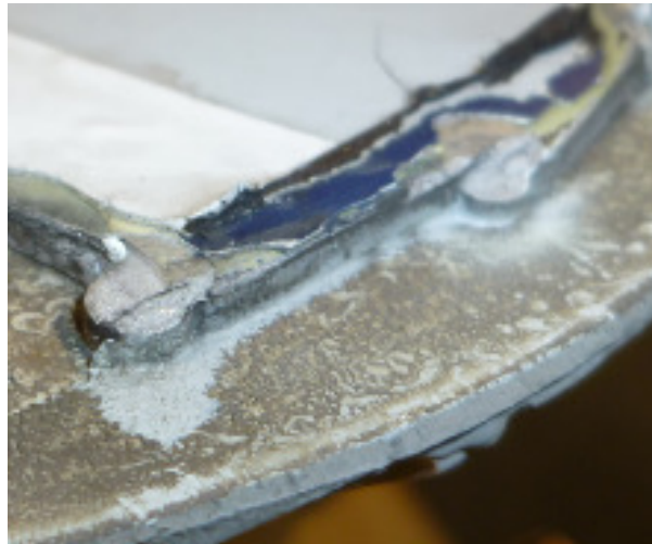
Figure 9: Paint seen under the door skin after seeping through existing door skin cracks
