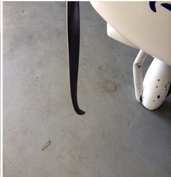
Figure 4: View of propeller damage
