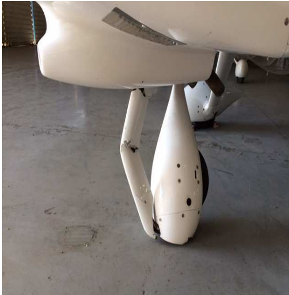
Figure 3: View of nose gear damage
