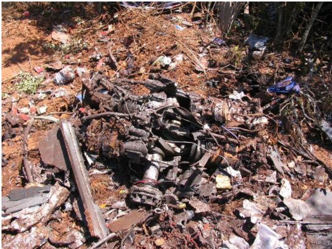
Figure 17: The engine which was severely deformed and split open
