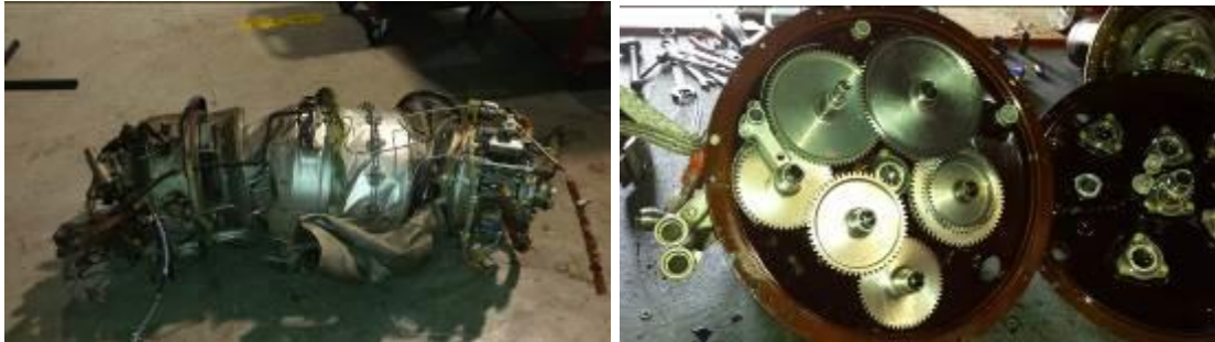
Figure 6: Left engine before and after teardown. The reduction gears had not been disturbed or affected.
