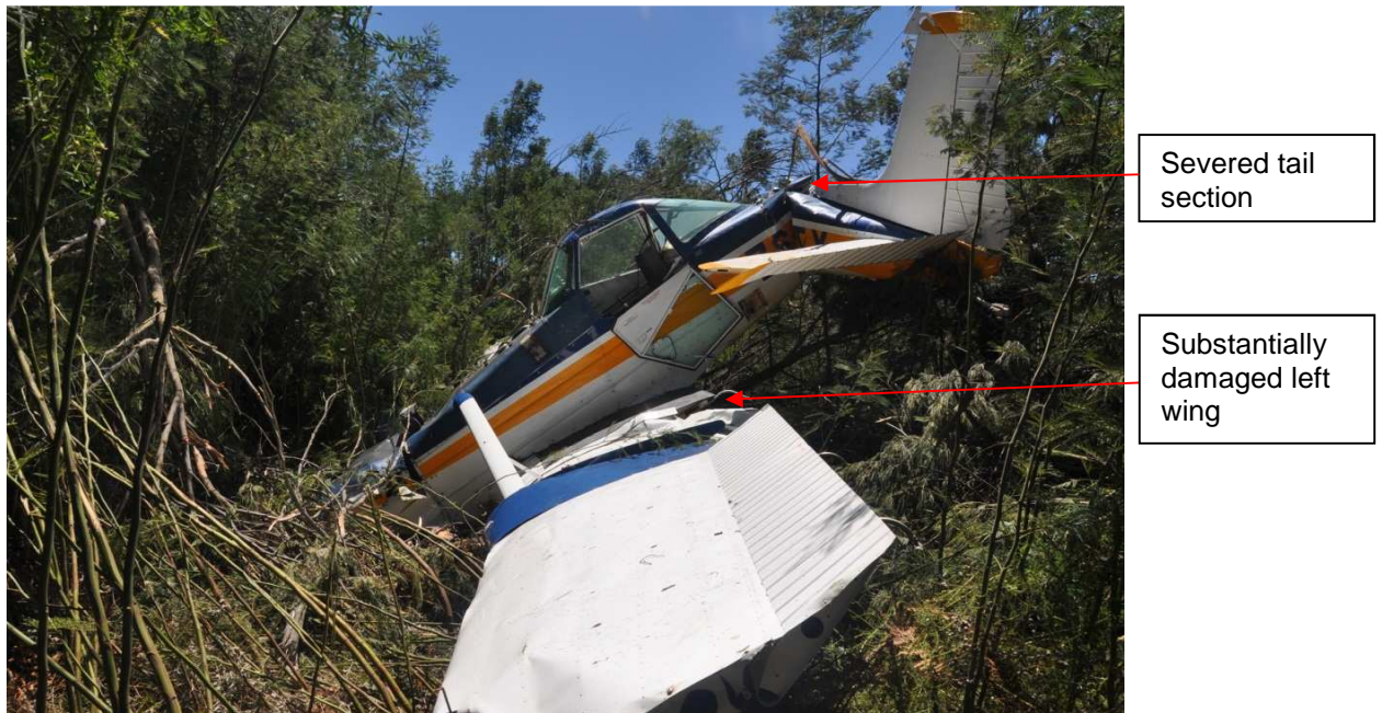
Figure 2: The wreckage as found at the accident site.
