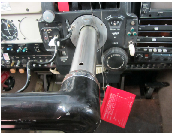
Figure 3: Position of levers in incident aircraft Figure 4: Position of controls in Beech Baron 58
