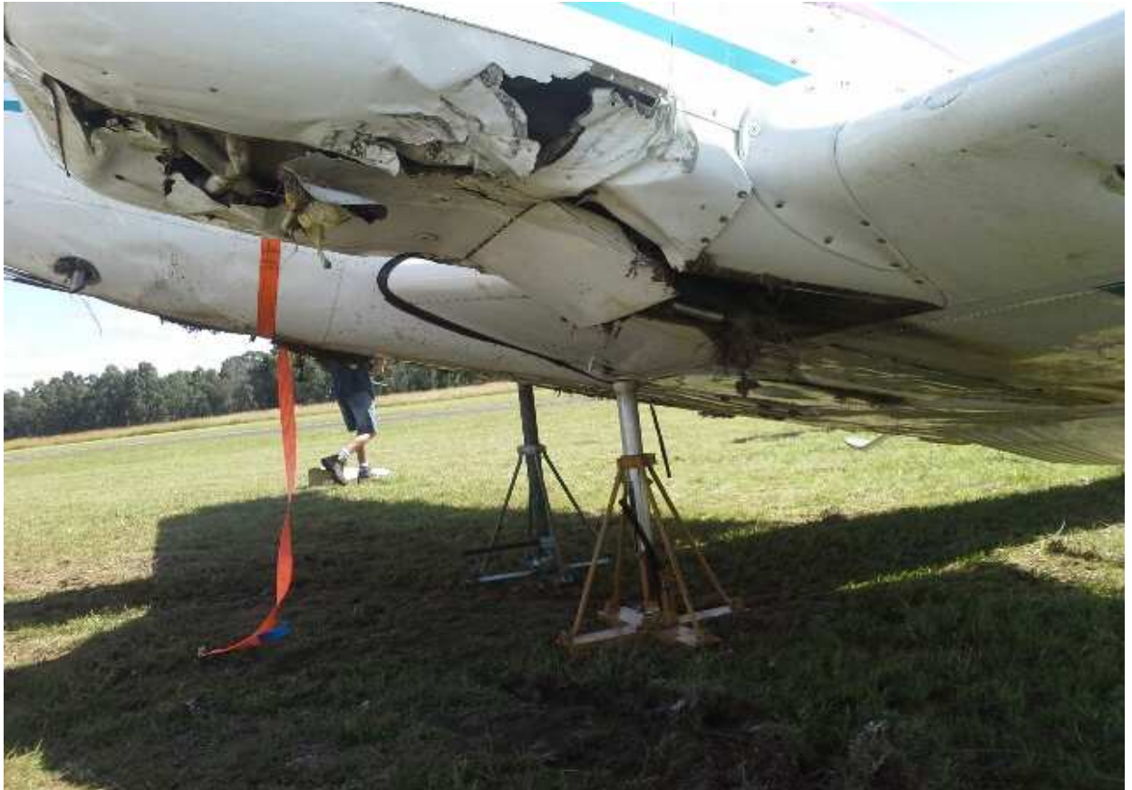
Figure 4: The damage to the aircraft surface
