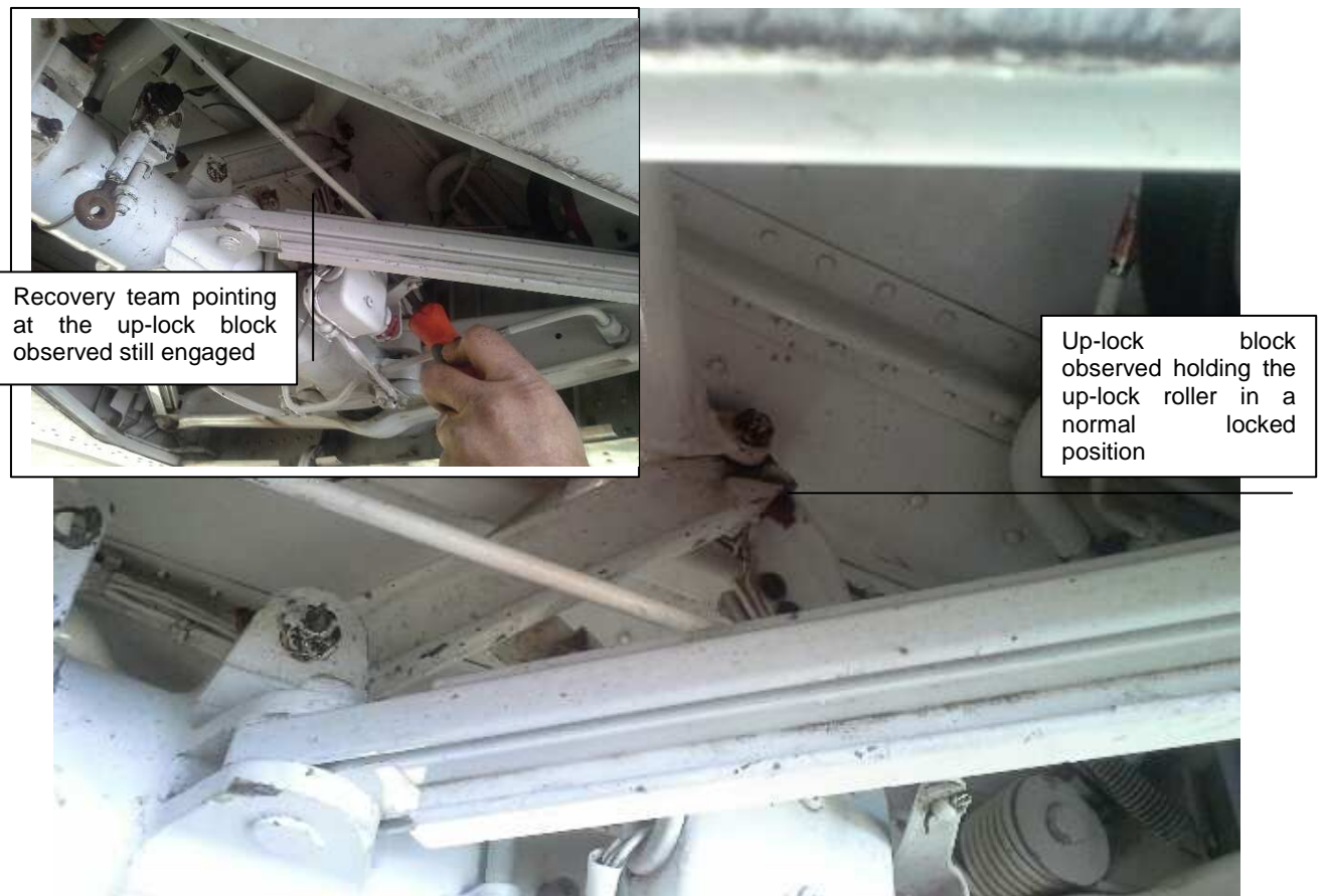
Figure 6: Up-lock stop bracket bolt installed from front to back
