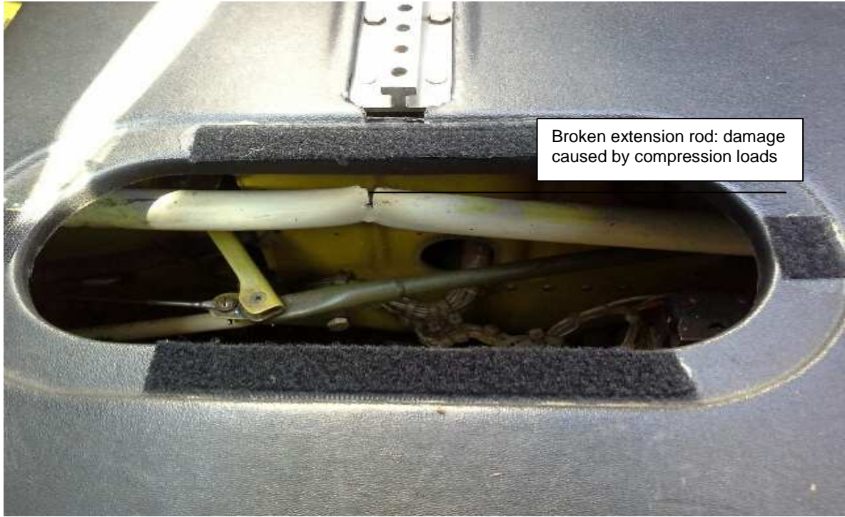
Figure 5: Damage to the landing gear extension rod
