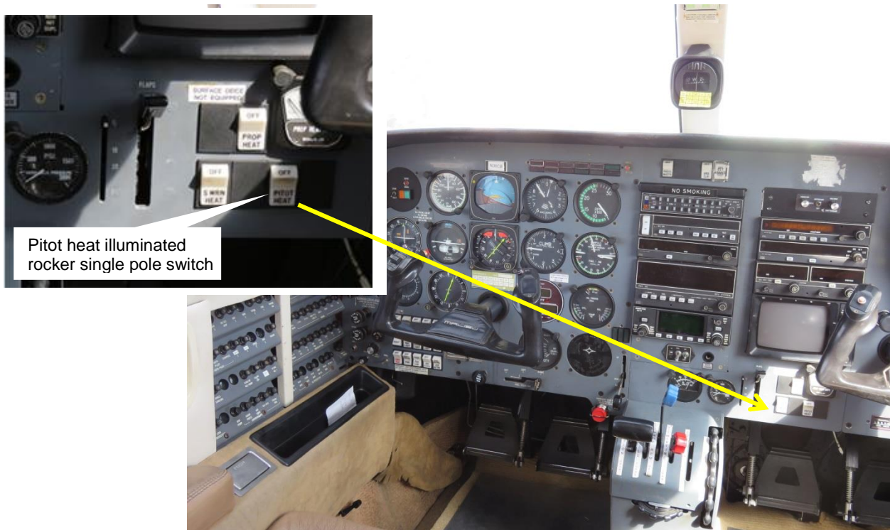
Figure 17 & Inset: Pitot heat switch in the cockpit on a similar aircraft
