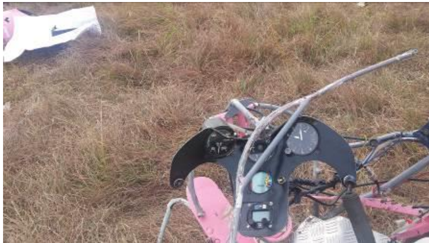
Figure 2: Damaged instrument panel and broken cockpit tubing.
