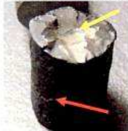
Photo 21: No 2 exhaust valve fracture surface, stem end (digital)
