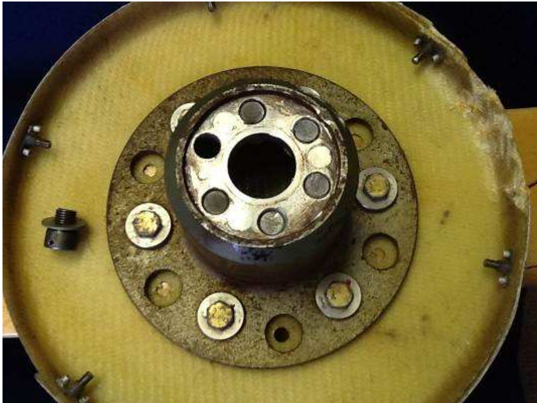
Figure 5. The sheared propeller attachment bolts (rear of the propeller)
