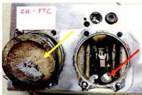
Photo 12: Engine block - No 2 piston damages (digital)
