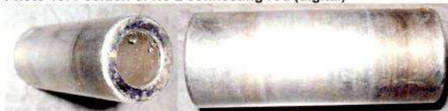
Photo 14: Gudgeon pin – small end No 2 (digital)
