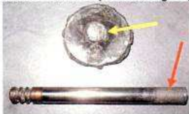
Photo 20: No 2 exhaust valve damages (digital)
