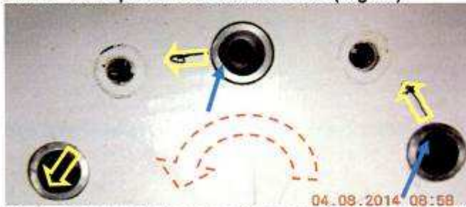
Photo 5: Impact damages to propeller bolt guides (digital)
