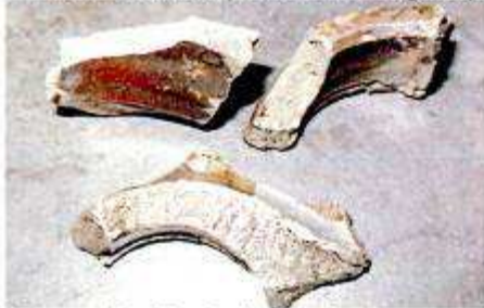
Photo 16: No 2 piston fracture surfaces (digital)
