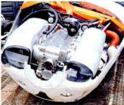
Photo 25: Similar failure of the propeller flange bolts following an engine failure (courtesy SACAA)
