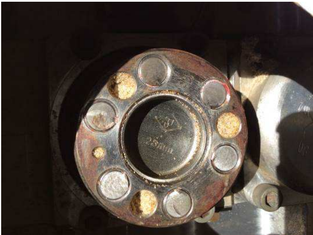
Figure 4. The sheared propeller attachment bolts (engine side).
