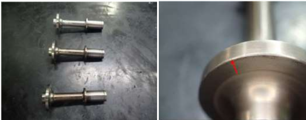
Burr at outer Diameter on all the three P 2.5/3 Air Switching Valve
