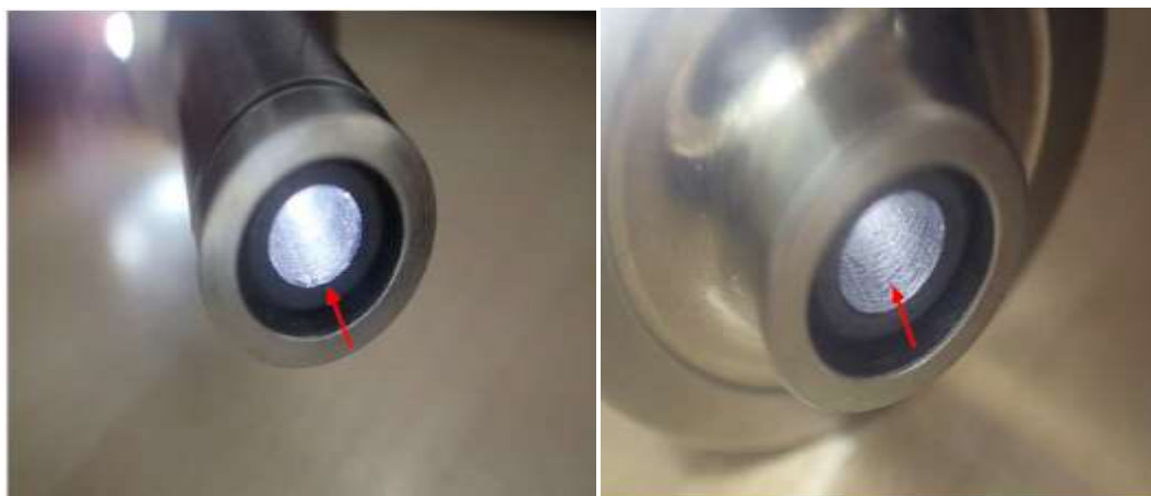
Wear in bushing inner diameter in two of the P 2.5/3 Air Switching Valve
