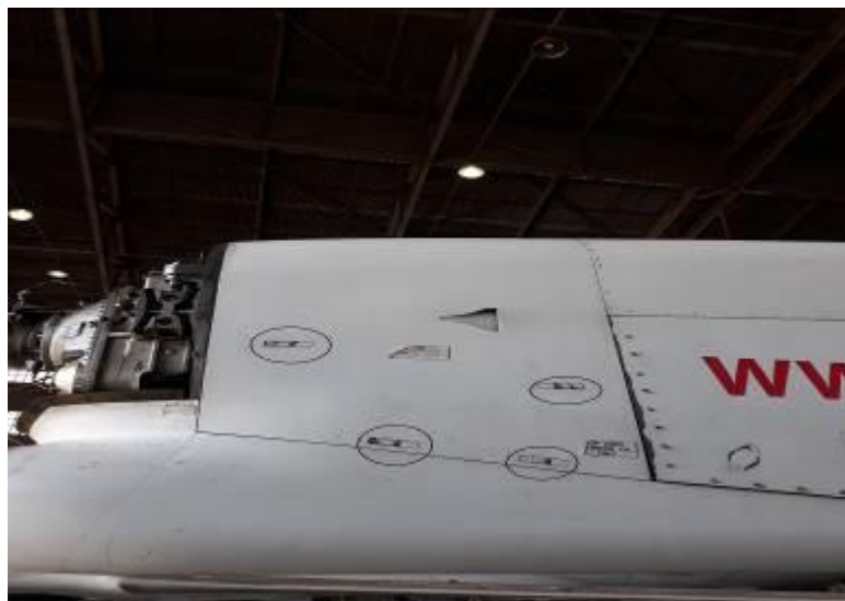
Figure 2: shows No 2 engine cowling position on a DHC-8-402
