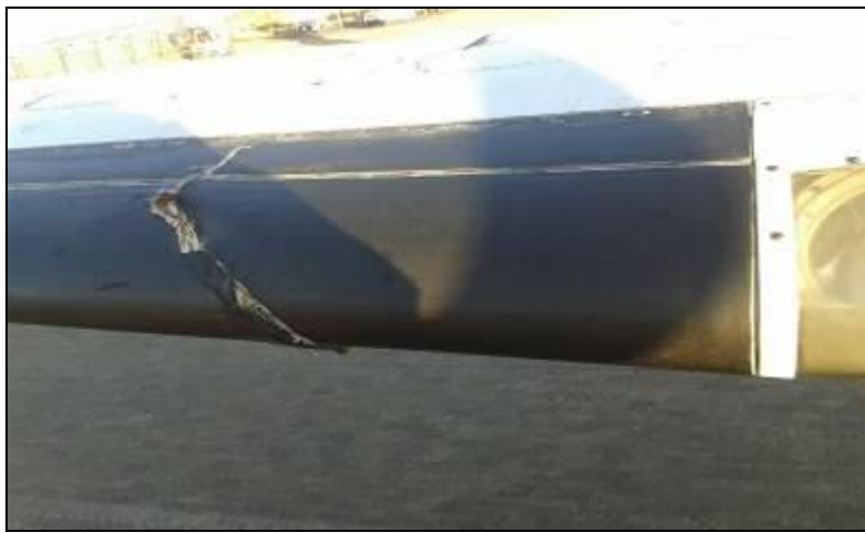
Figure 1: Shows R/H leading edge & de-icer boot damaged
