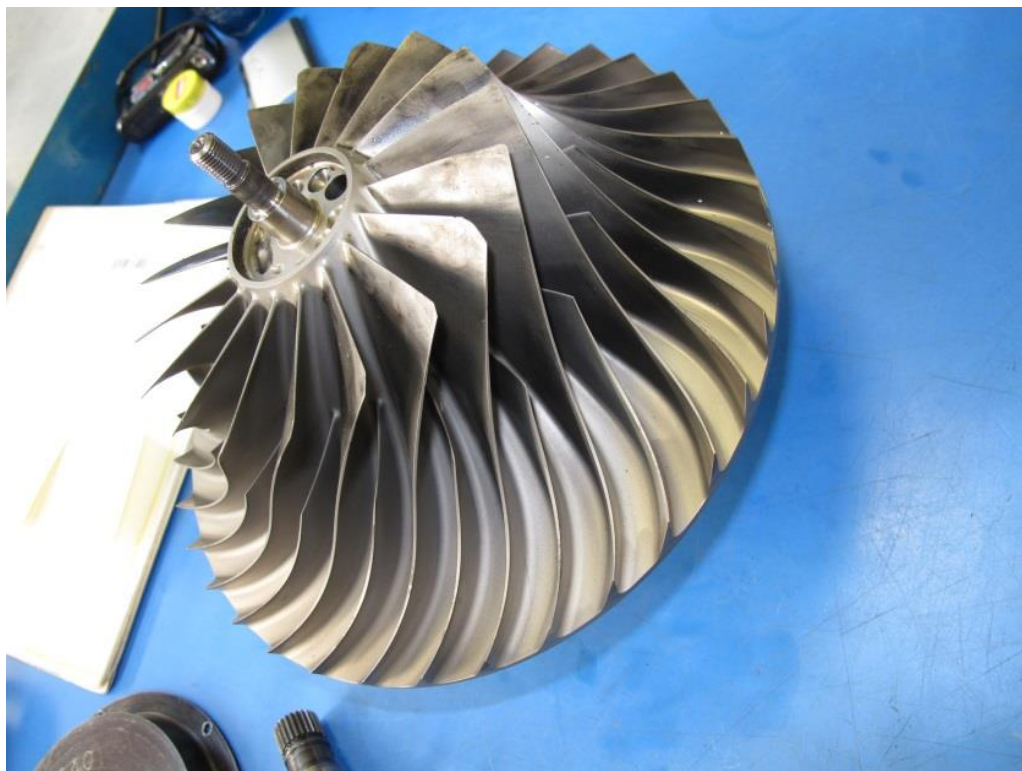
Figur 12. Radialkompressor i gott skick.
