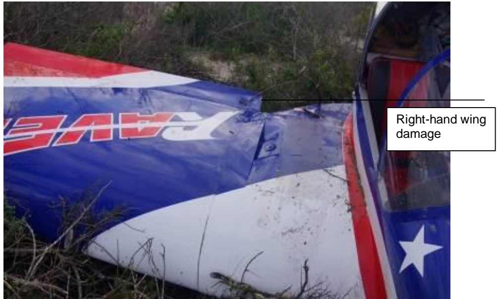
Figure 4: Damage to the right wing
