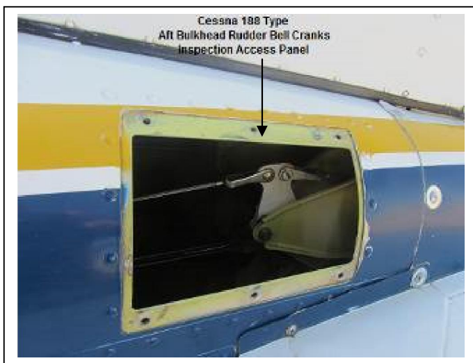
Figure 4 & 5 Example of access panel and bell crank installation in a similar type of aircraft
