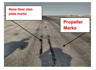
The intensity of the impact on the nose gear on the runway was so strong that both the fork link of the nose wheel broke due to impact on the runway. The nose wheel went away and the propeller hit the runway surface at about 1020 metres from threshold.
