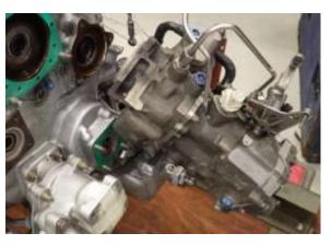
The AGB fuel pump pad was found with broken studs. Engine teared down.
