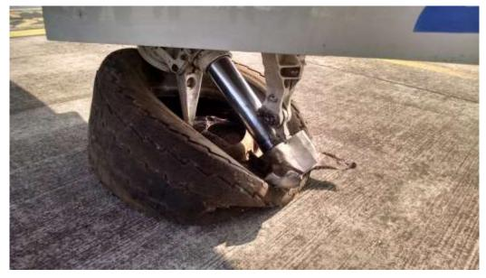
NOSE LANDING GEAR BENT BACKWARD
