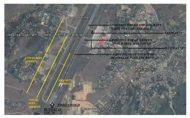
Figure: Location of aircraft and parts on the runway after landing.
