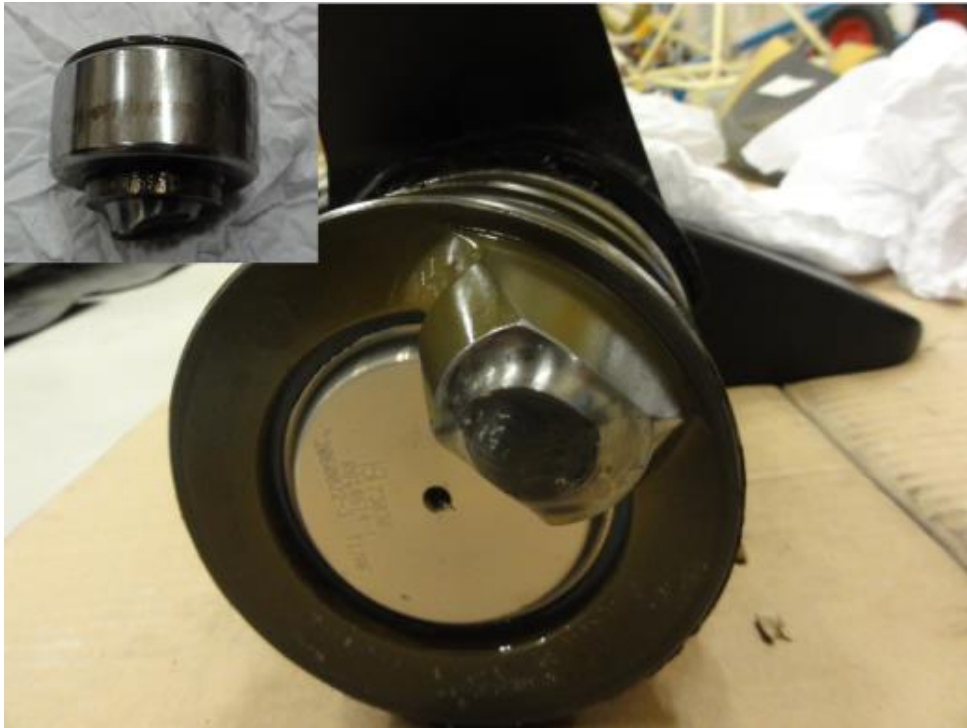
Figure 3. The ruptured eccentric trunnion pin.
