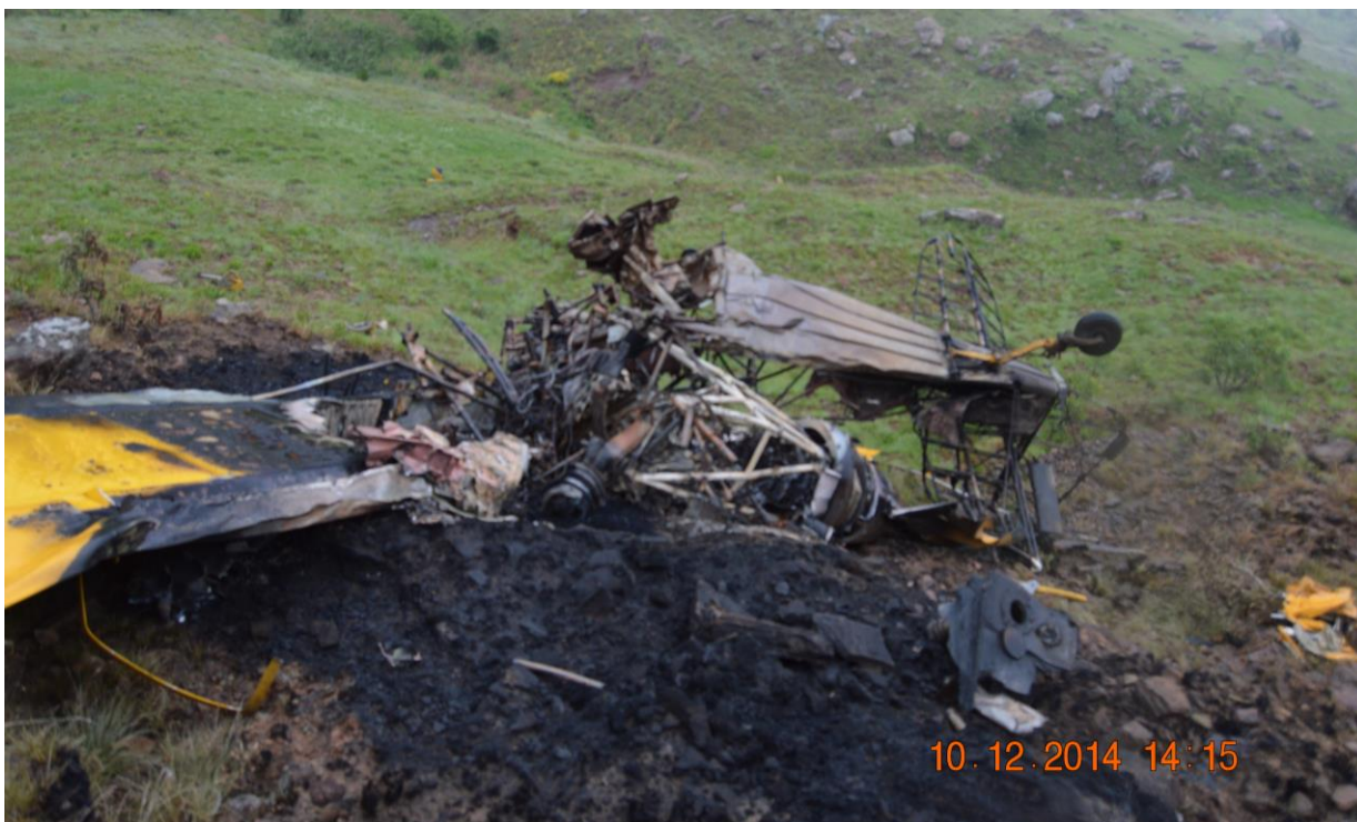
Figure 3: Mangled and burnt ZS-LJT airframe
