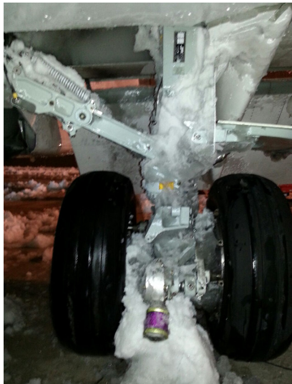
Photograph 1. Condition of the gear the night before the incident
