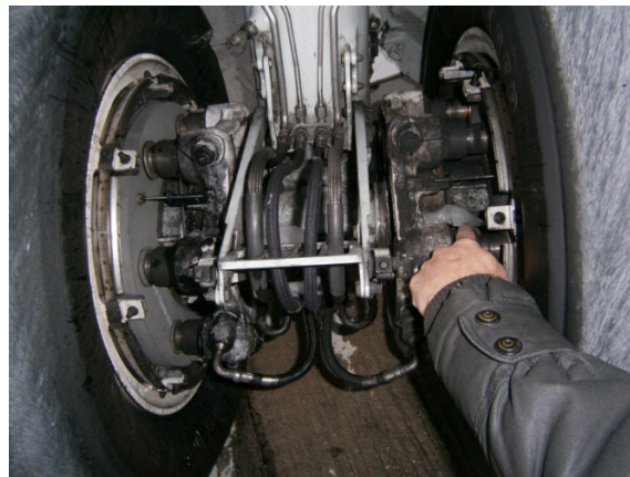
Photograph 3. Blocks of ice still adhering to the brake assemblies
