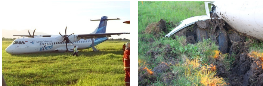
Figure 8: The nose landing gear collapsed rearward and damaging the front lower fuselage
