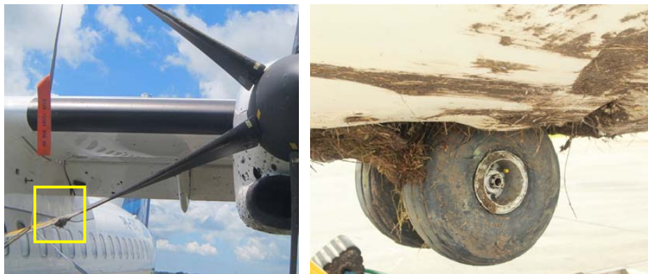
Figure 4: The damage on the propeller and the nose wheel
