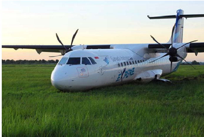
Figure 3: The final position of the aircraft with the nose and main landing gears trapped on the soft soil
