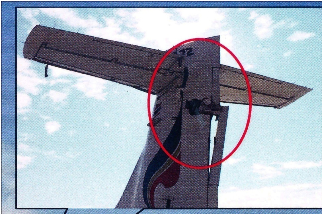
Figure 5. The damaged vertical stabilizer of Bangkok Airways Aircraft
