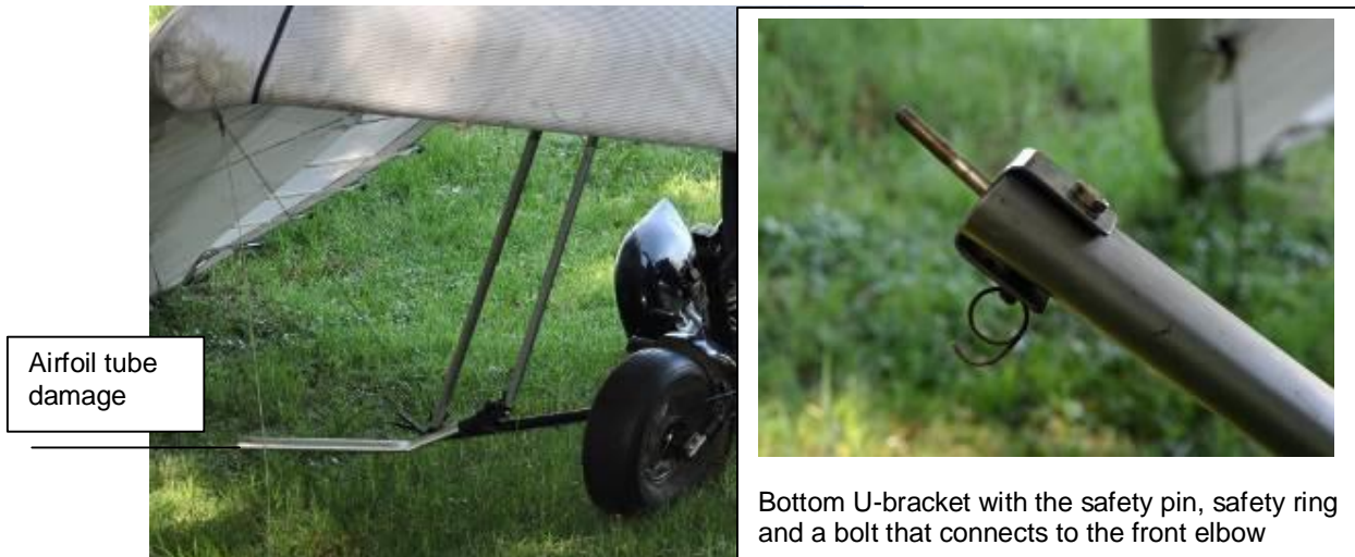
Figure 5: Airfoil with bottom U-bracket
