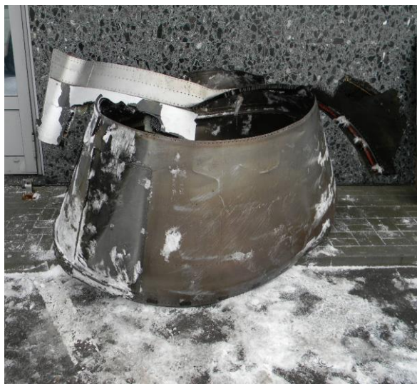
Figure 1. Aft right engine thrust reverser
