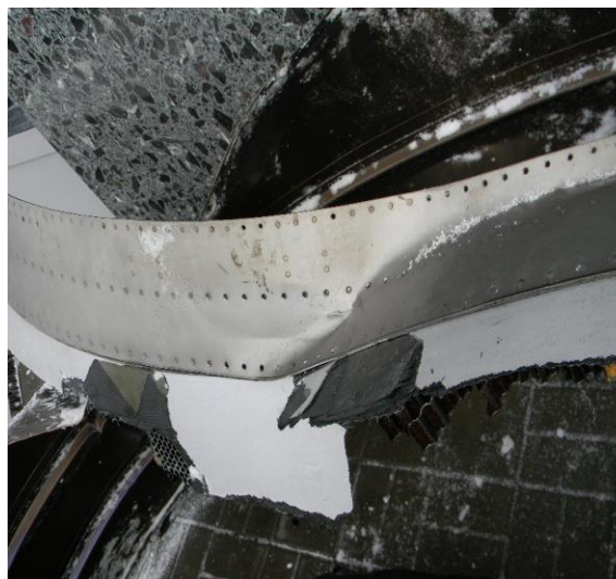
Figure 2. Detail of the aft thrust reverser
