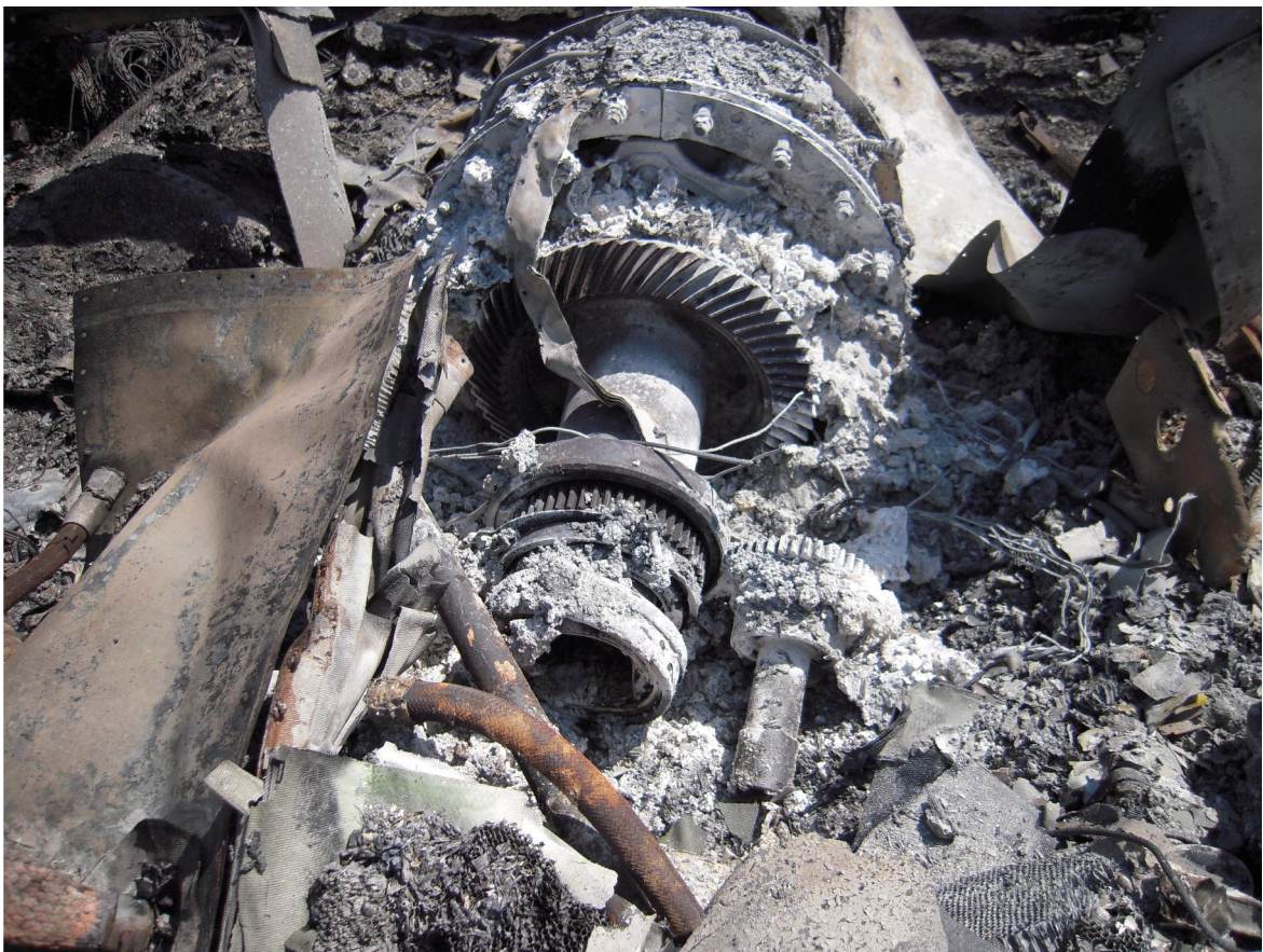
Figure 6. The main rotor gearbox consumed by the post-impact fire
