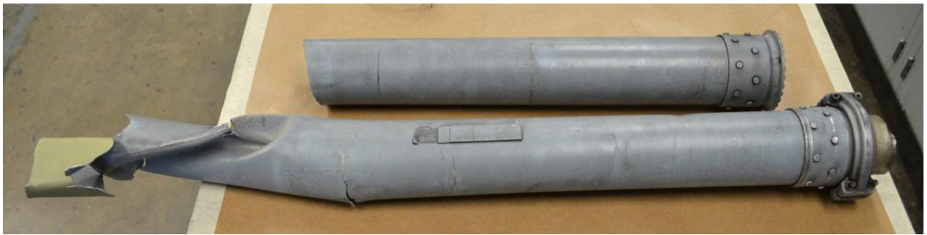
Figure 32. The twist direction on the tail rotor driveshaft indicates a sudden rotational stoppage aft of the twist.
