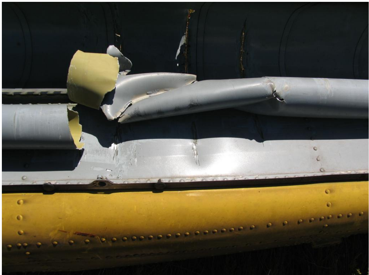
Figure 13. A closer view of the failed tail rotor driveshaft
