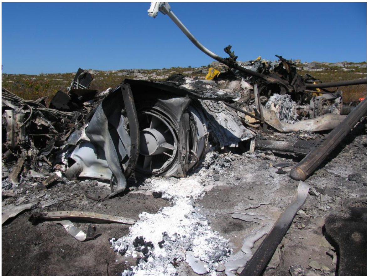
Figure 7. Aft section of the engine and main wreckage
