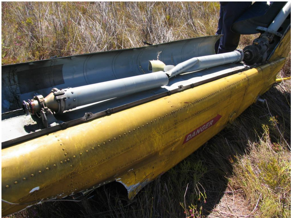
Figure 12. Tail rotor driveshaft just forward of the 42° intermediate gearbox fractured in torsional overload
