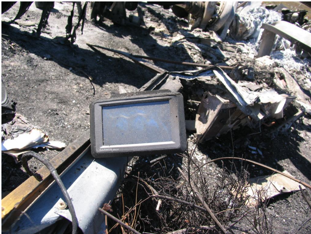
Figure 35. The damaged Garmin Aera 500 GPS (taken during the on-site investigation)
