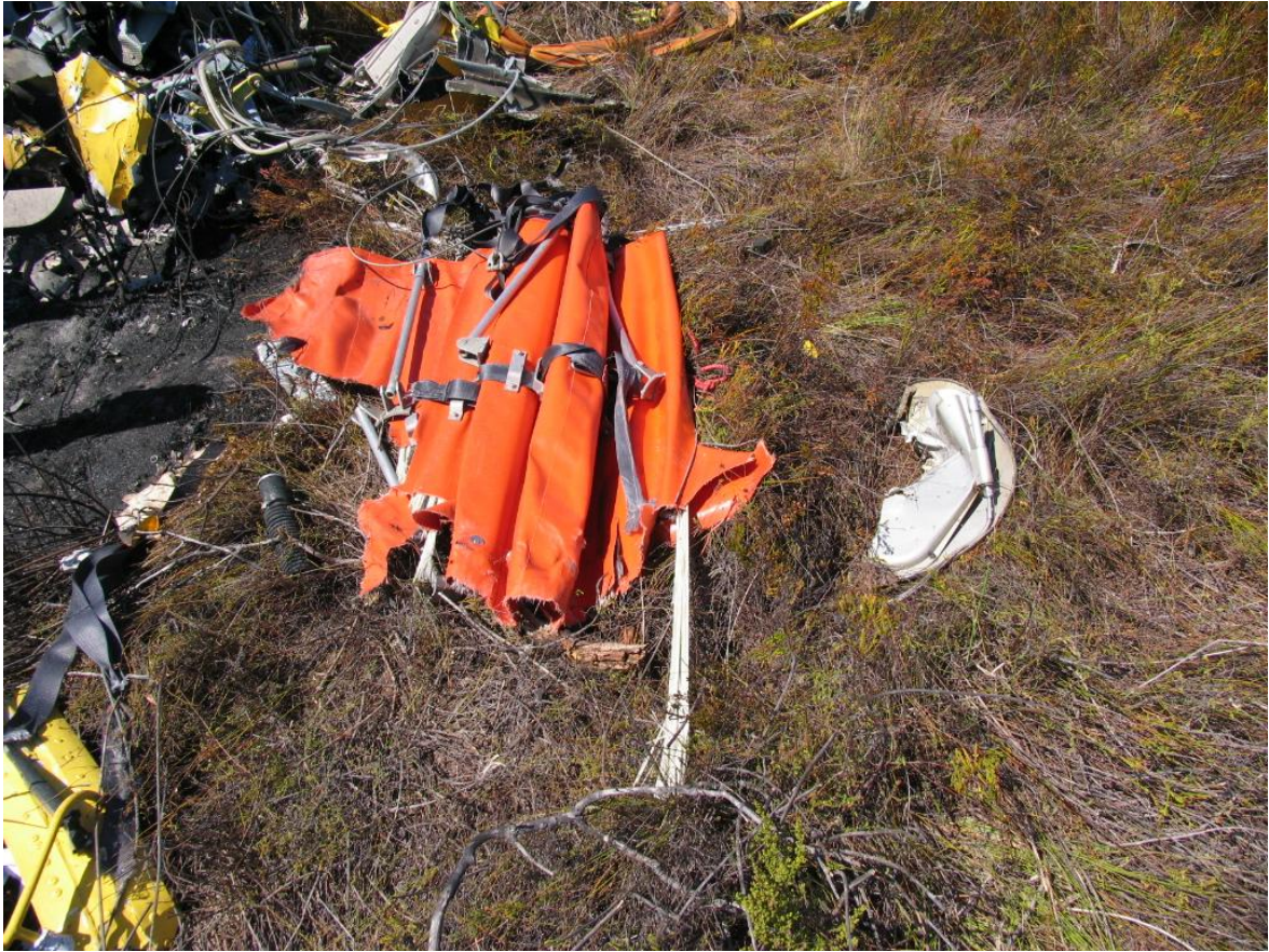
Figure 8. A section of the Bambi bucket that was severed by the main rotor blades
