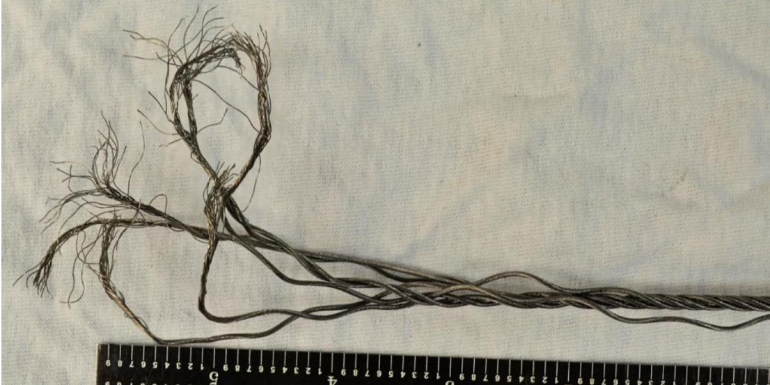
Figure 24. Fractured forward right-hand control cable
