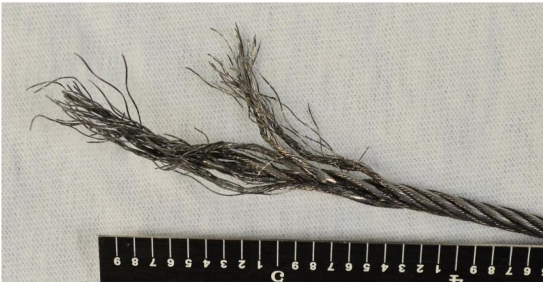
Figure 25. Fractured aft left-hand control cable
