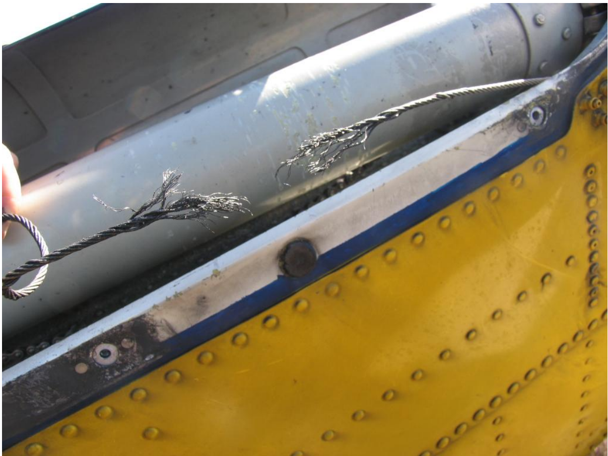
Figure 14. Photograph of both ends of the aft tail rotor control cable that was found to have failed
