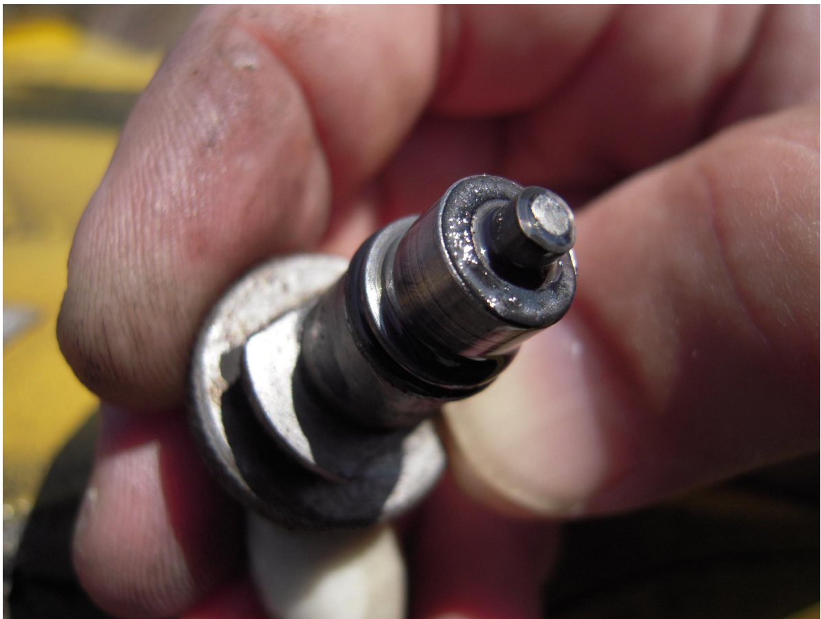
Figure 17. Magnetic plug on the 90° tail rotor gearbox removed during the on-site investigation
