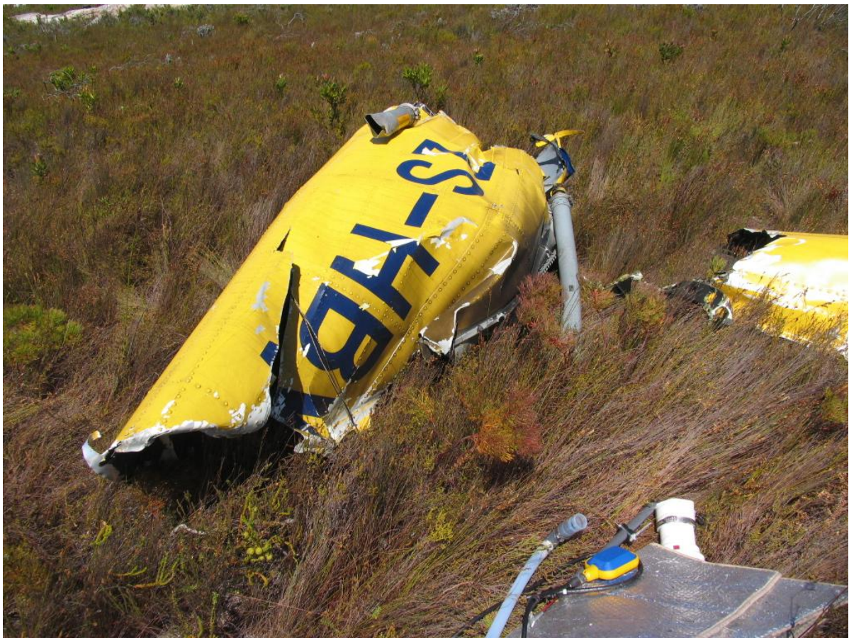
Figure 10. The forward tail boom structure that was severed by the main rotor blades
