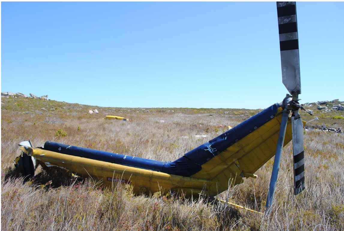
Figure 9. Aft tail boom and blades (tail boom was placed in an upright position)
