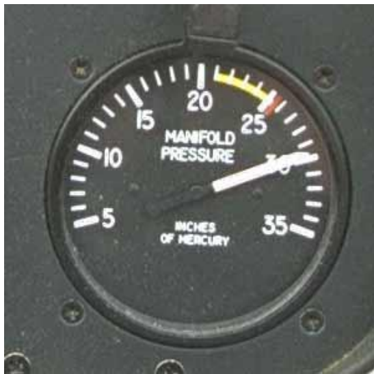
Figure 4: The manifold pressure gauge
