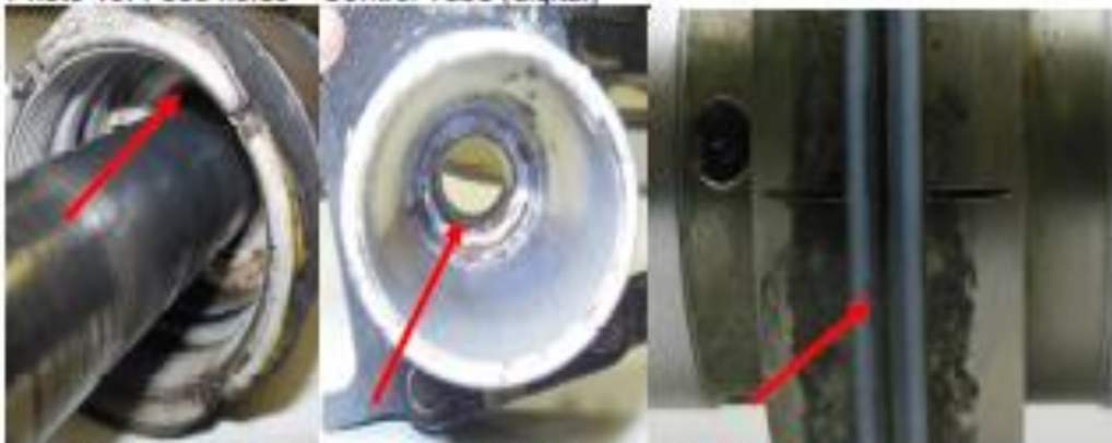
Photo 20: Hydraulic seal conditions – 3x positions – Control Tube (digital)
