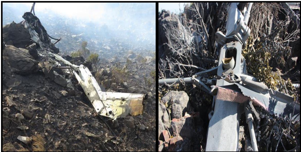
Figure 9: The damaged tail boom and tail rotor blade respectively.
