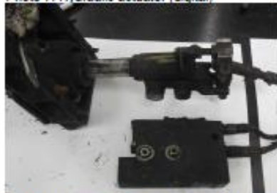
Photo 8: Hydraulic actuator - removed (digital)
