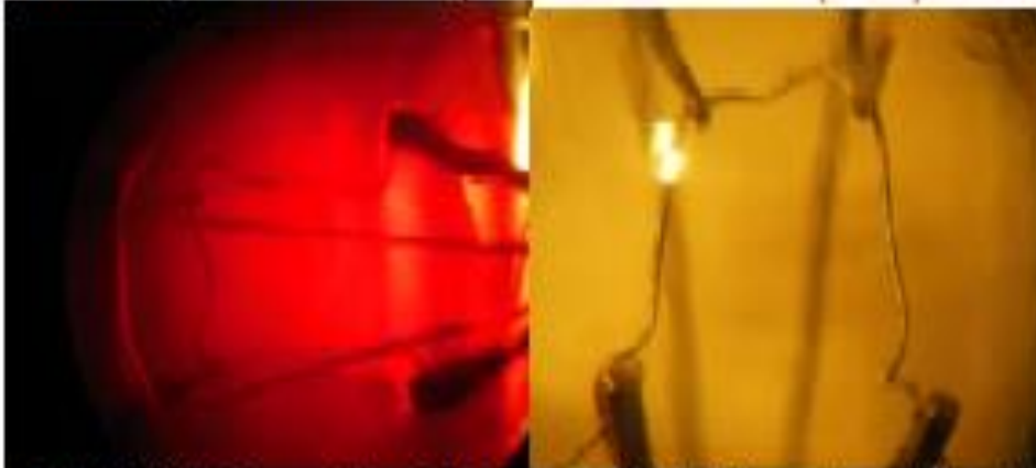
Photo 26: Main Transmission Oil Pressure - light bulb filament condition (stereo)
