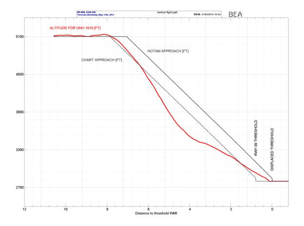
The flight safety office of the Airbus Co. also performed a vertical flight path computation which has similar results.
