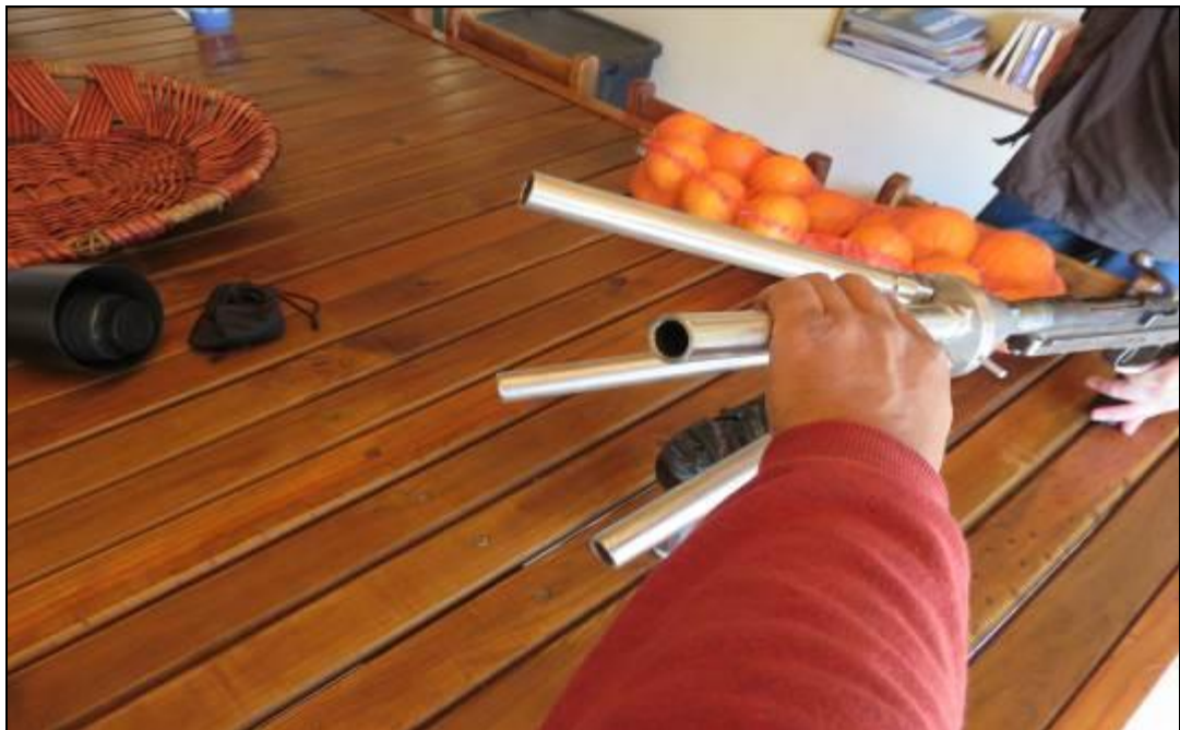
Figure 4: The net-gun displayed with the four barrels where the weights are fired from
