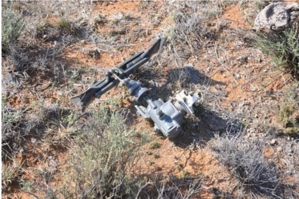
Figure 3: The tail rotor gearbox, hub and two severed stubs tail rotor blades
