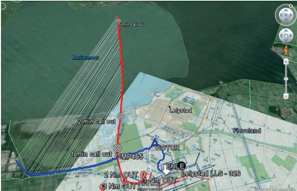
Figure 4: Flight path of Dornier aircraft with call out positions and distances in NM from runway threshold on extended centreline. For orientation, the top of the page is north and the bottom of the page is south.
