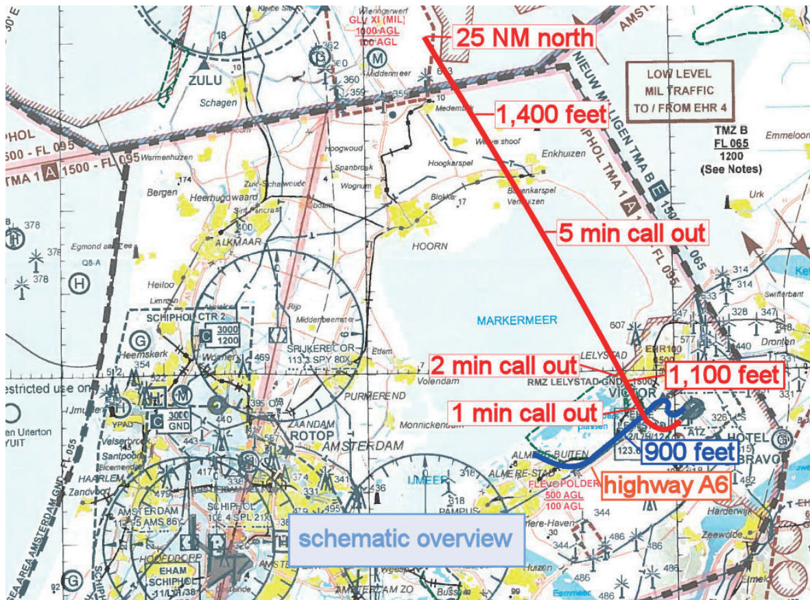
Figure 1: Aeronautical Chart ICAO, The Netherlands: D-IROL in red and PH-4D3 along highway A6 in blue.
