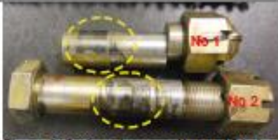
Photo 10: Surface damages, No1 and 2 bolts (digital)
