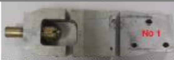
Photo 5: Sectioned No MR Blade attachment bracket (digital)
