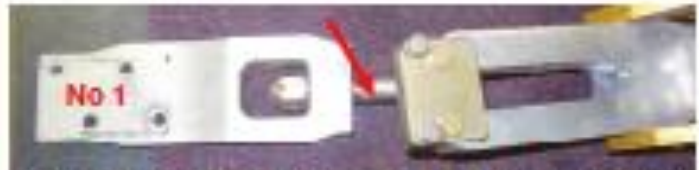
Photo 3: Position of fractured No 1 MR blade attachment bolt (digital)
