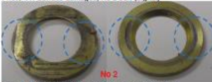
Photo 12: Washer, bolt head end, No 2 bolt (digital)
