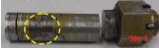
Photo 6: Surface damages, No 1 bolt, sectioned (digital)
