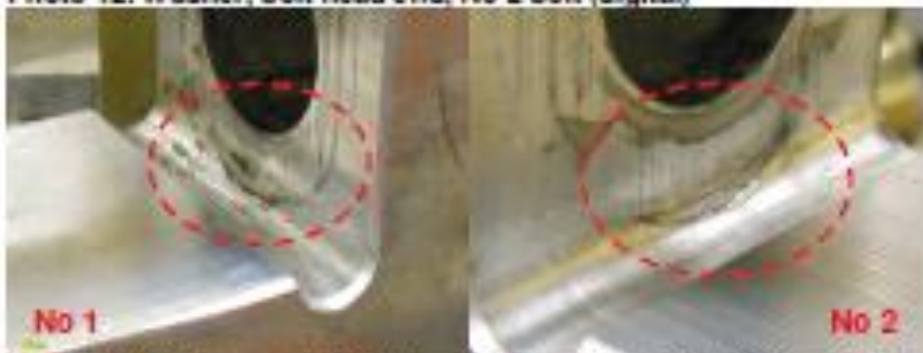
Photo 13: Washer and MR blade attachment bracket interface, No 1 and 2 bolts (digital)
