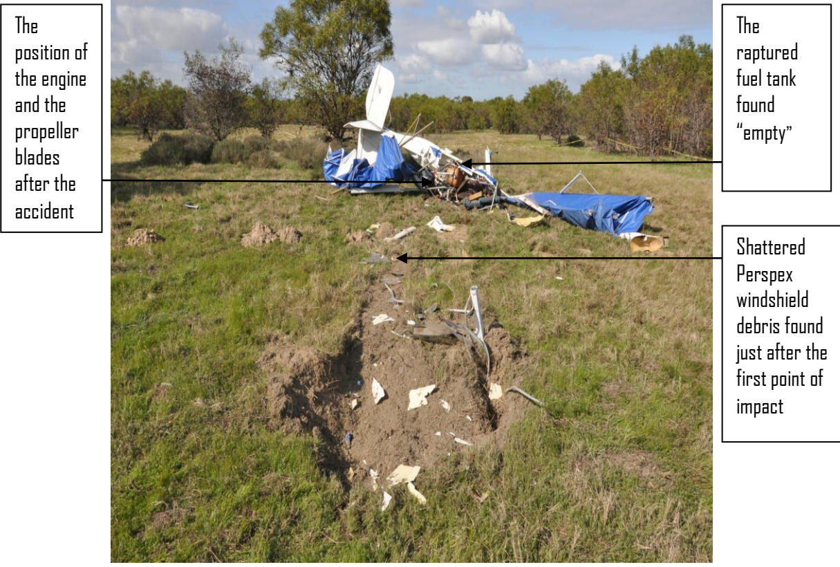
Figure 7: The aircraft first point of impact and the final position of the wreckage
