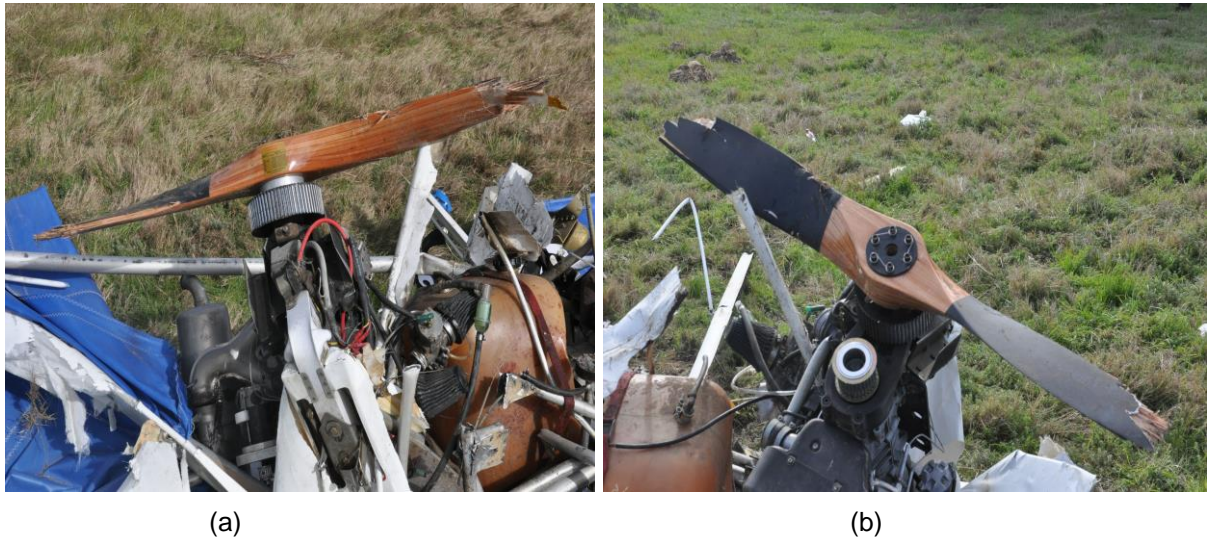
Figure 10: The propeller was attached to the engine and displayed tip damage; indicating that the engine had been providing power at the moment of impact
