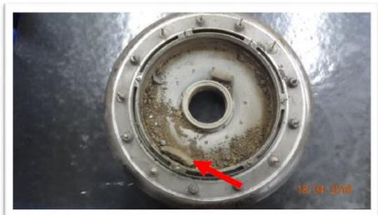
Image #14: Indications of soil ingestion noticed on the 1st Stage Diffuser.
