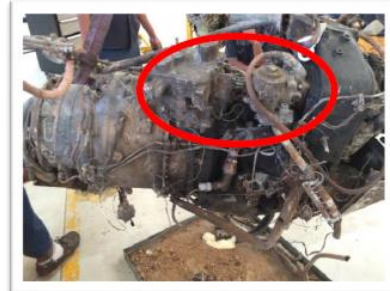
Image #2: The F.C.U. was noted to have broken off the Fuel Pump Assembly at F.C.U. – Fuel Pump split line.
