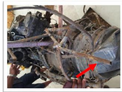
Image #4: The Exhaust Duct was noted to be bent severely.
