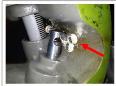
Image #10: The nuts and retaining studs securing the Output Housing Seal Carrier were found sheared within the Output Housing.
