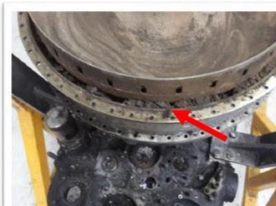
Image #12: Further indications of soil ingestion were noted between the Compressor Housing and the Outer Transition Liner.
