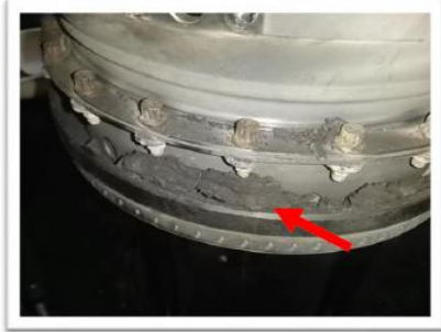
Image #16: Indication of soil ingestion noted within the Inner Transition Liner.
