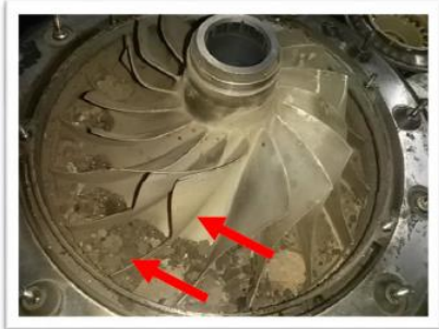
Image #13: Numerous vanes of the 1st Stage Impeller were found to be bent severely. Indications of soil ingestion found between the vanes.
