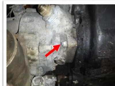
Image #8: The run-off torque was very low on most of the fasteners.
