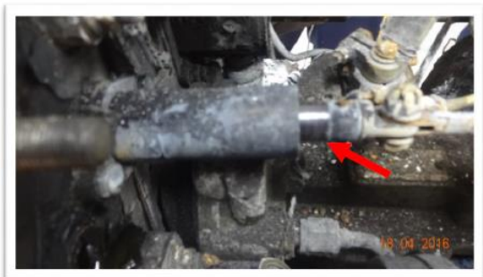
Image #19: The Feathering Valve did not appear to have been stroked at disassembly.
