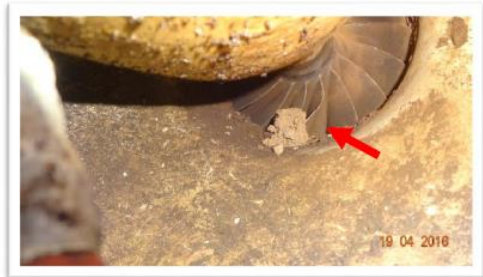
Image #6: Deposits of soil found within the engine intake. Numerous vanes on the 1 st Stage Impeller are damaged.
