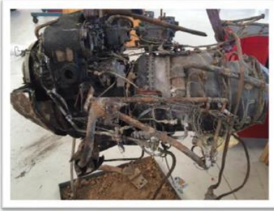
Image #1: The dark deposit/discolouration on the engine is indicative of exposure to fire.
