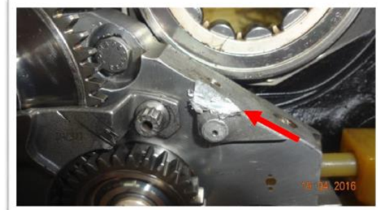
Image #18: Abnormal wear noted on the Torque Sensor body.
