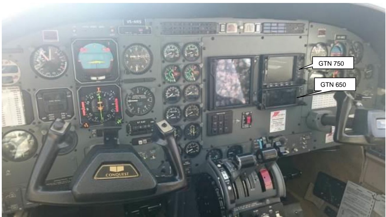
Figure 5: Installation of the GTN 750 and GTN 650 GPS in the accident aircraft
