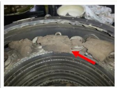
Image #11: Indications of soil ingestion were noted between the Combustion Chamber and the Combustion Liner.
