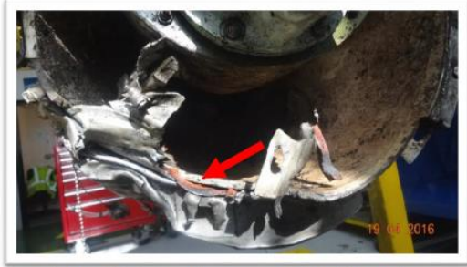
Image #3: Severe damage noted to the engine intake.
