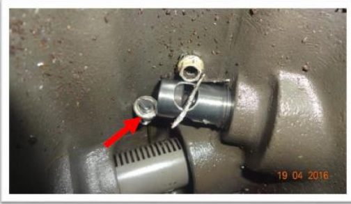
Image #13: Remains of retaining studs and nuts from Output Housing Carbon Seal Carrier found in bottom of Output Housing.
