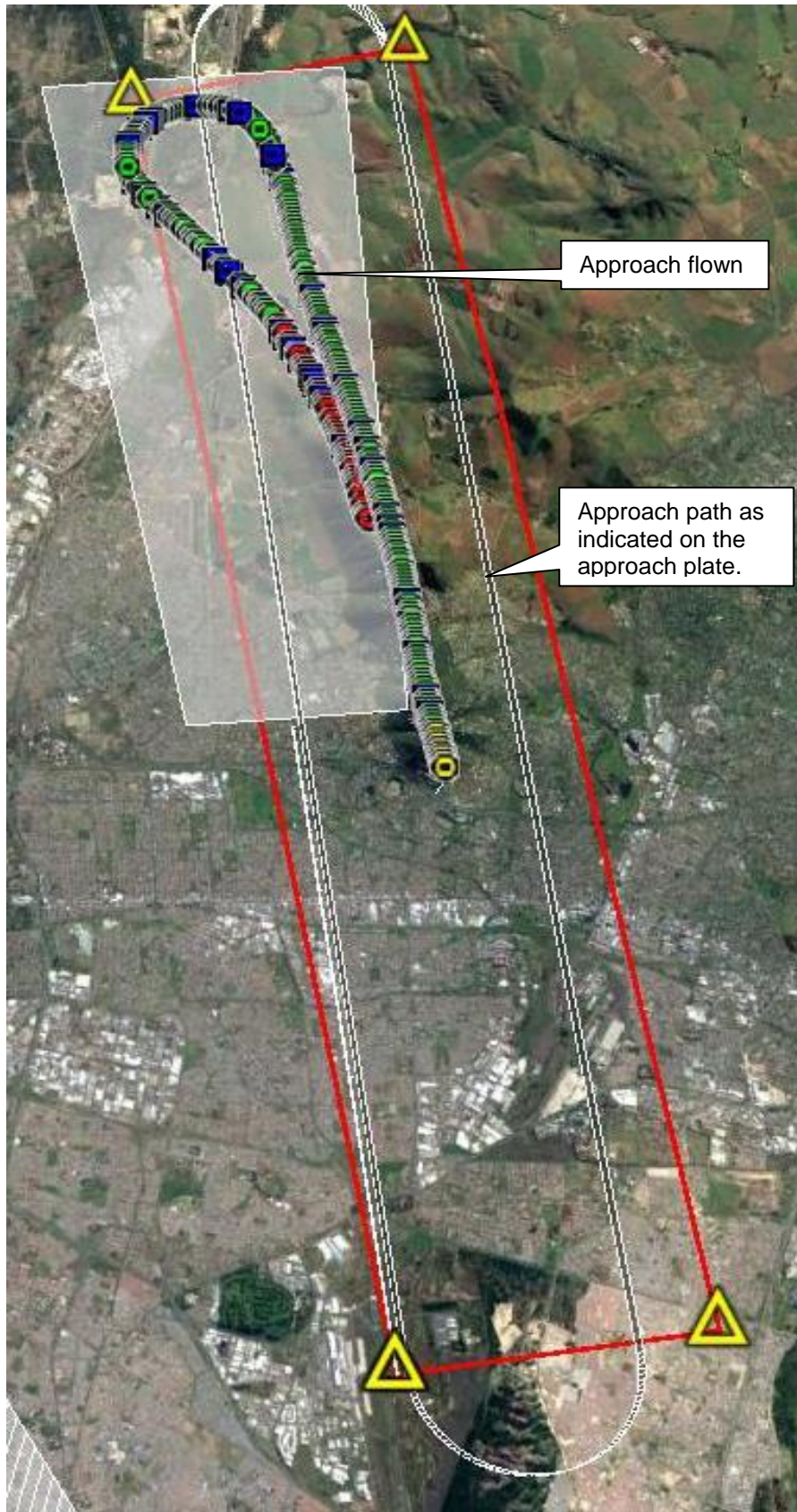
Figure 9: Reconstruction of the profile flown by the crew during the approach
