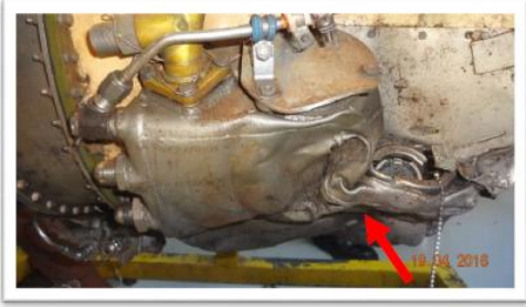
Image #9: Oil Tank appears to be crushed.
