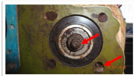
Image #8: Fuel Pump Assembly mounting studs missing from Accessory Housing. Splined drive shaft was noted to be sheared.
