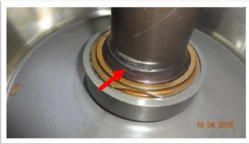
Image #15: Abnormal wear noted on Propeller Shaft, possibly caused by rub from the Sun Gear.
