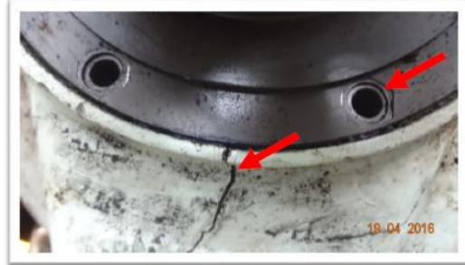
Image #4: Output Housing severely damaged. Retaining studs on Output Housing Carbon Seal carrier are missing.
