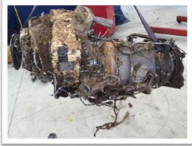
Image #1: Severe impact damage was noted on numerous components of the engine.
