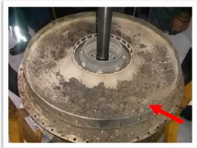
Image #15: Indications of soil ingestion noted on the Outer Transition Liner.
