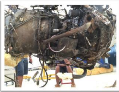
Image #3: Most externally mounted components were burnt and/or severely damaged.
