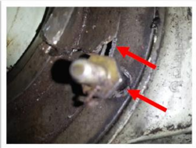
Image #9: The Output Housing Carbon Seal Carrier was noted to be cracked severely. Also, the retaining studs were noted to be missing or migrated forward.
