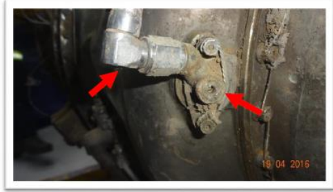
Image #10: Sections of the fuel manifold and fuel nozzles were broken off.
