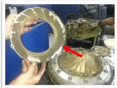
Image #14: Indications of soil ingestion noticed on the 1st Stage Shroud. No Impeller to Shroud contact noted.
