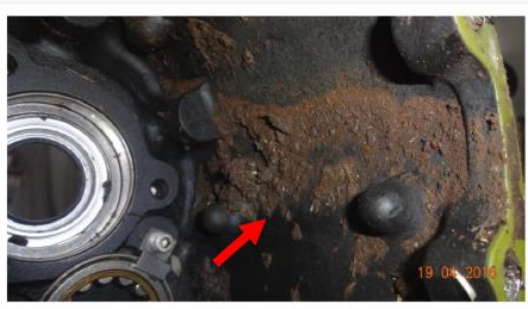
Image #19: Indications of soil deposits within the Accessory Housing.
