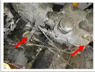
Image #5: Upon disassembly of the engine it was noted that the P.P.C. and F.C.U. protractors were possibly indicating the cockpit power lever position to have been at 60 degrees Power Lever Angle.
