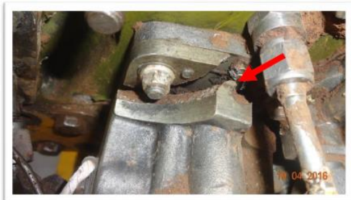
Image #7: Propeller Governor found parted from the mounting pad.
